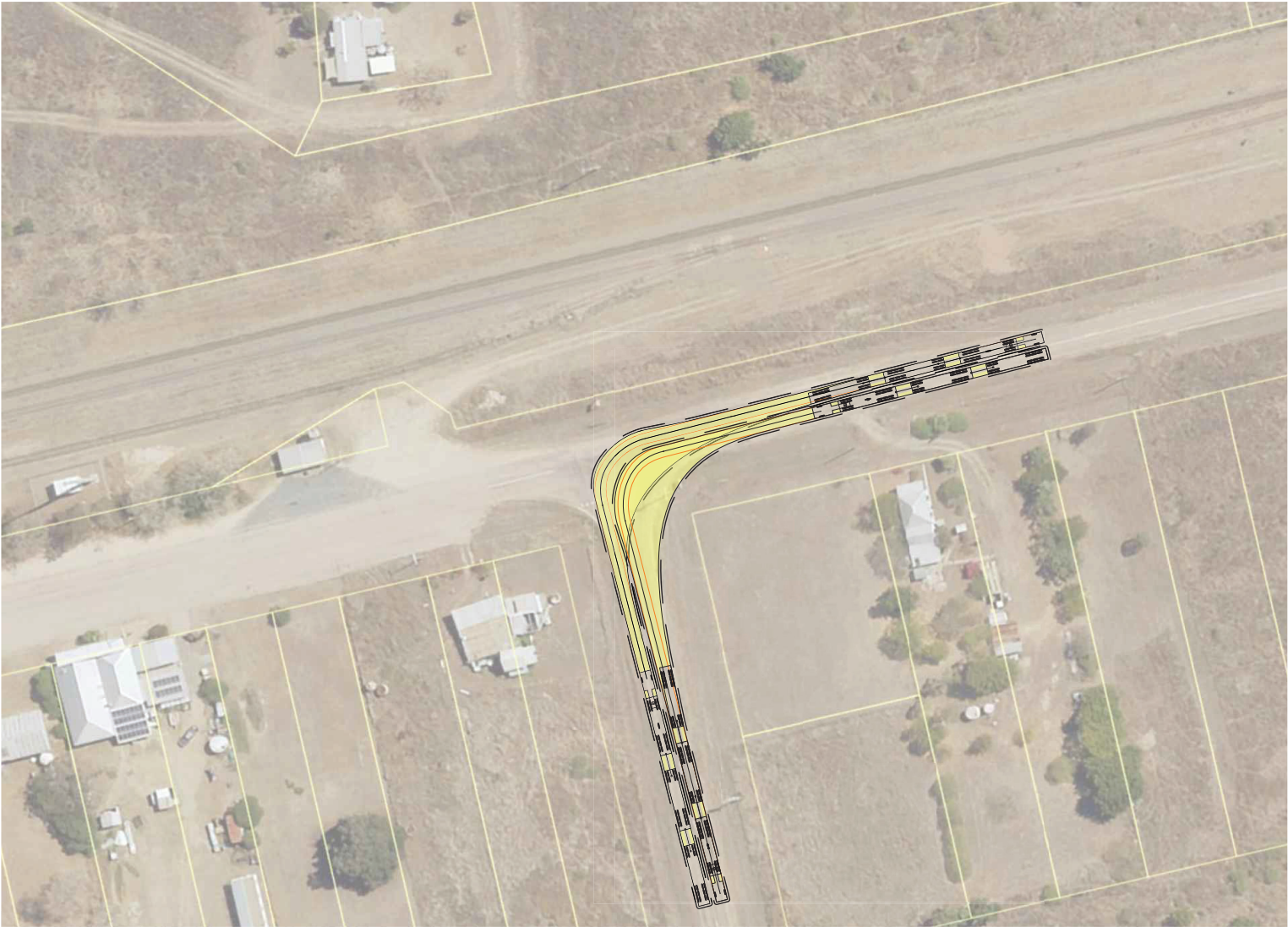
A TRIPLE SWEEP PATHS - TMR02 SCALE 1:500
