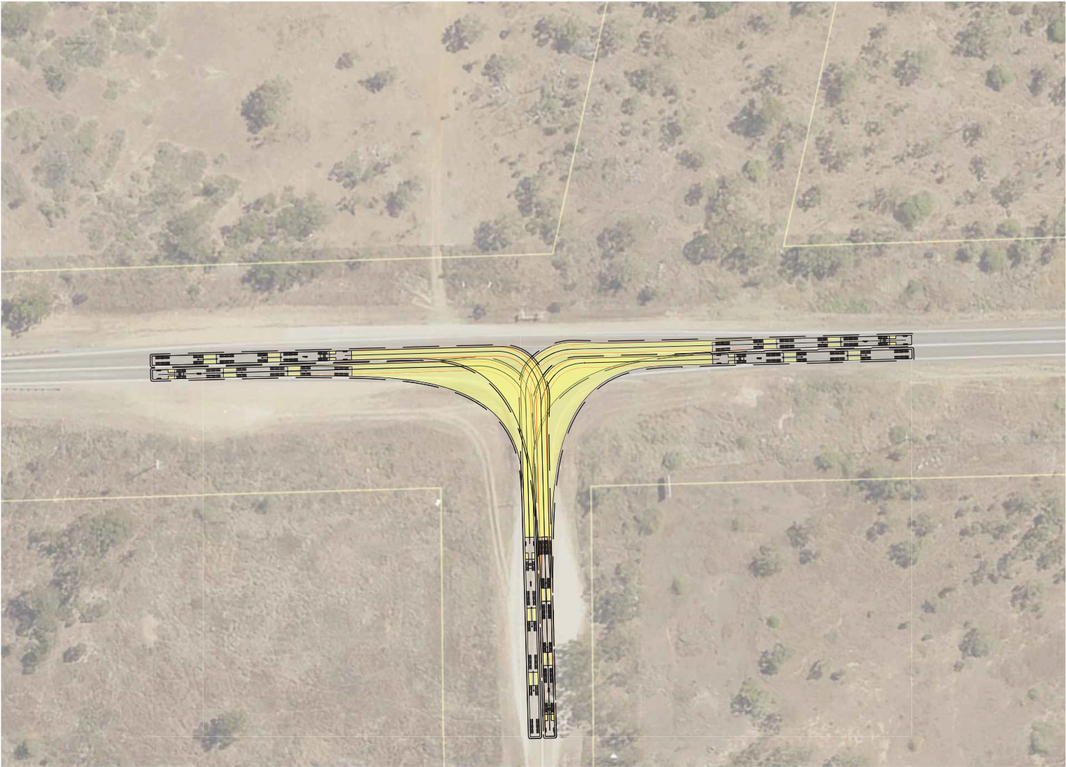
A TRIPLE SWEEP PATHS - TMR01 SCALE 1:500
