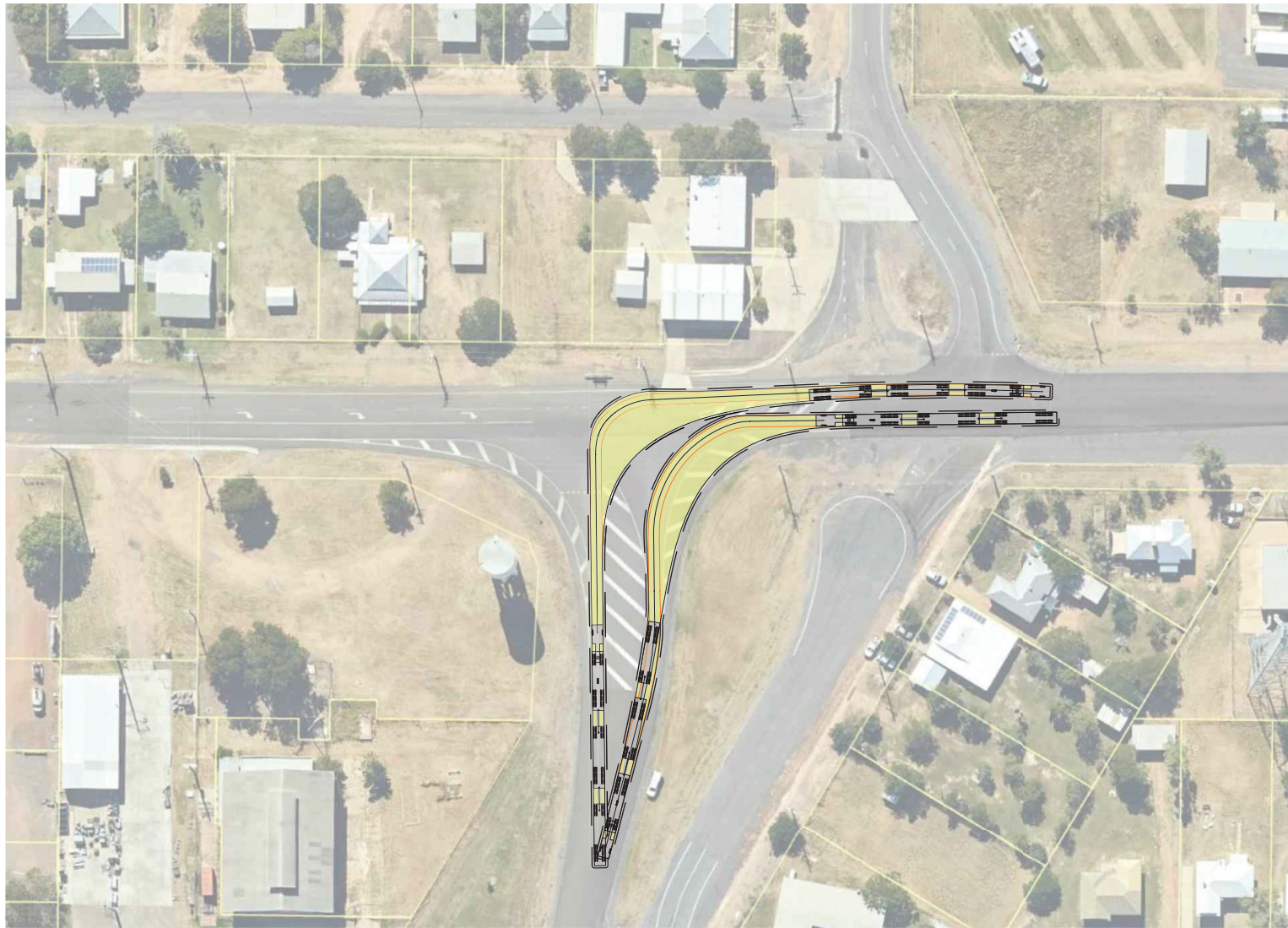
A TRIPLE SWEEP PATHS - TMR14 SCALE 1:500
