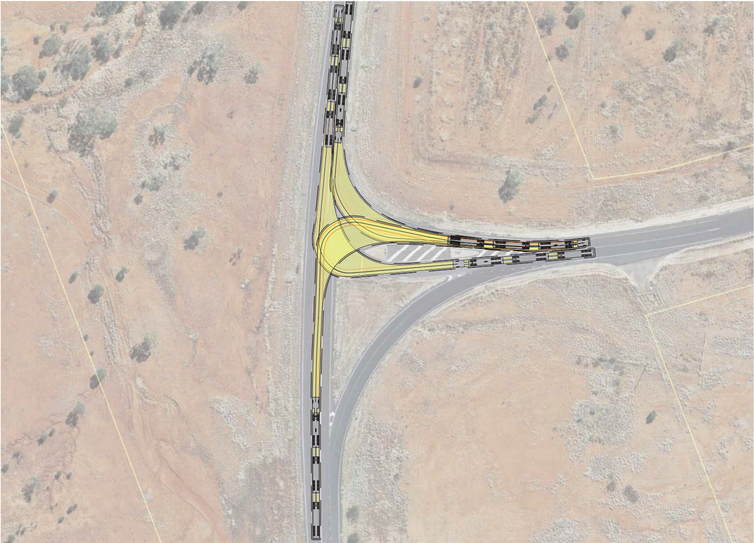
A TRIPLE SWEEP PATHS - TMR37 SCALE 1:500
