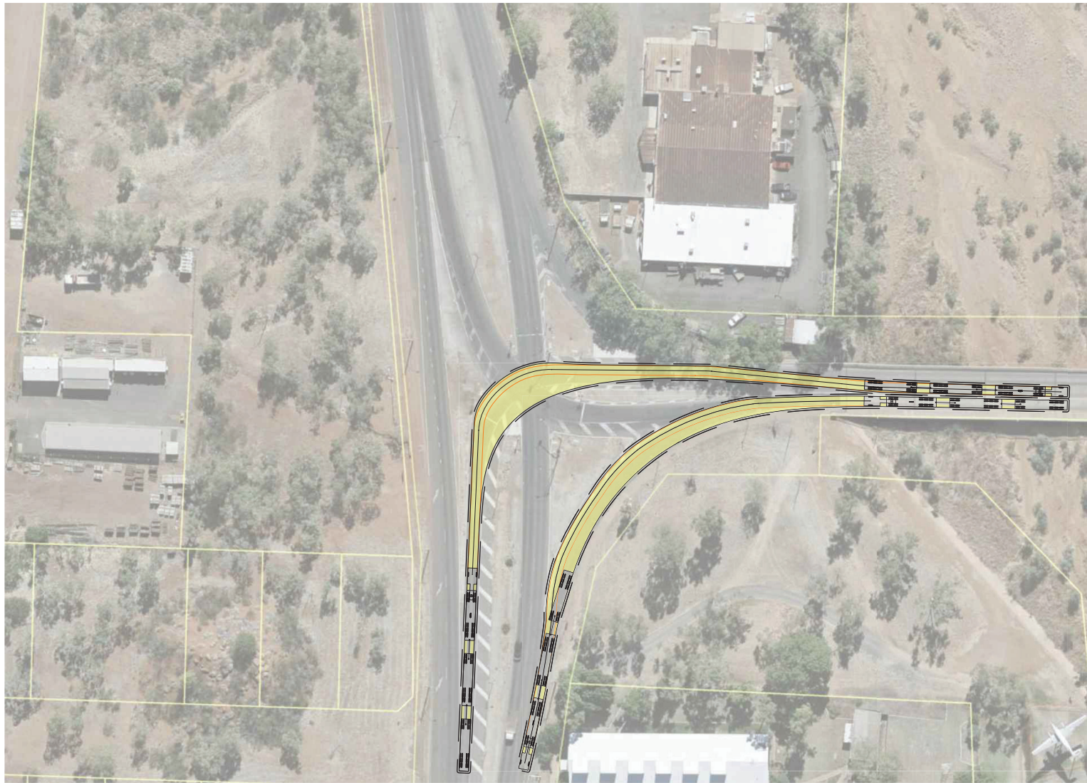
A TRIPLE SWEEP PATHS - TMR33 SCALE 1:500
