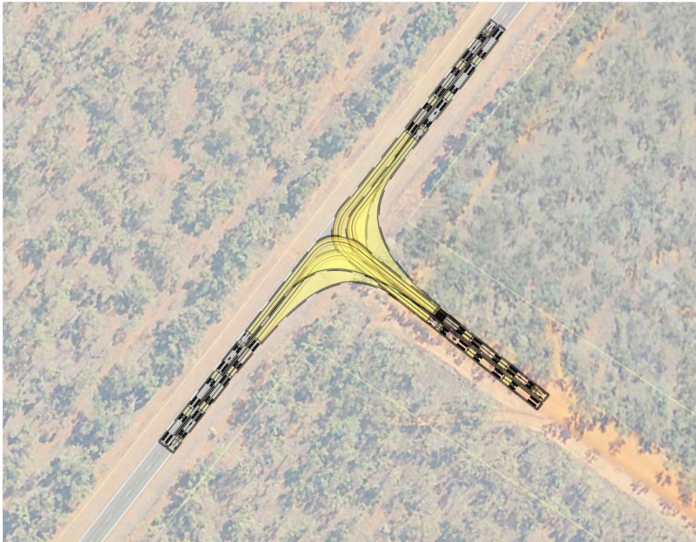
Figure 4-1 Local government intersection turn path example
