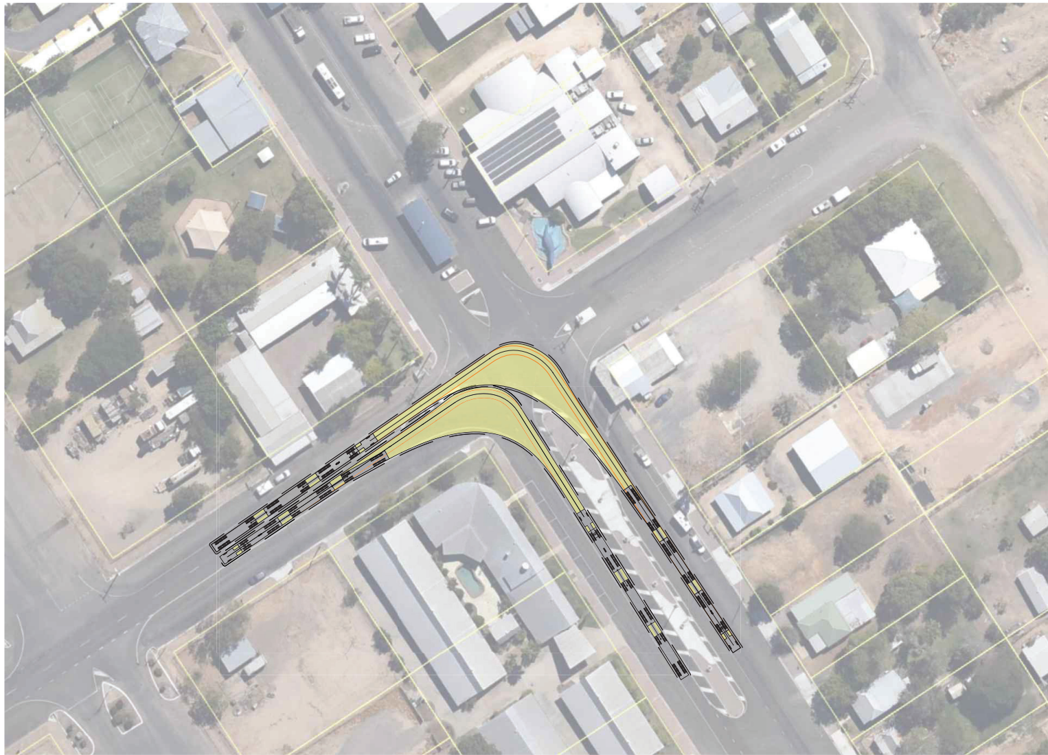
A TRIPLE SWEEP PATHS - TMR16 SCALE 1:500
