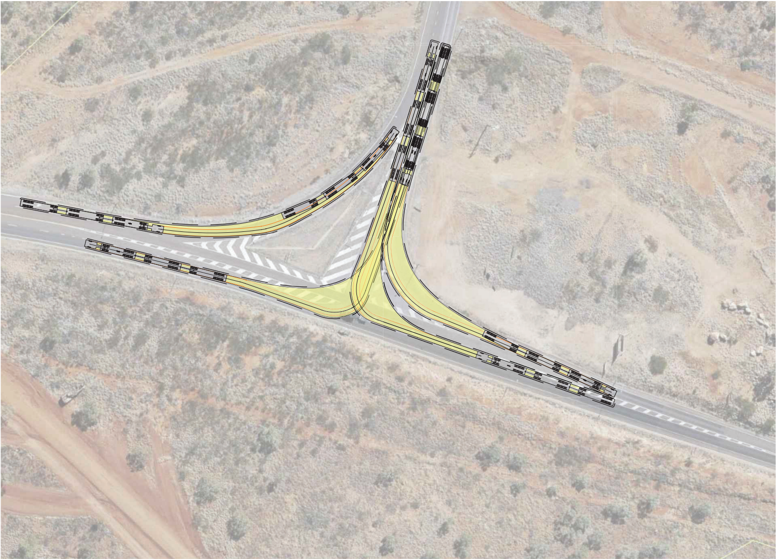
A TRIPLE SWEEP PATHS - TMR36 SCALE 1:500
