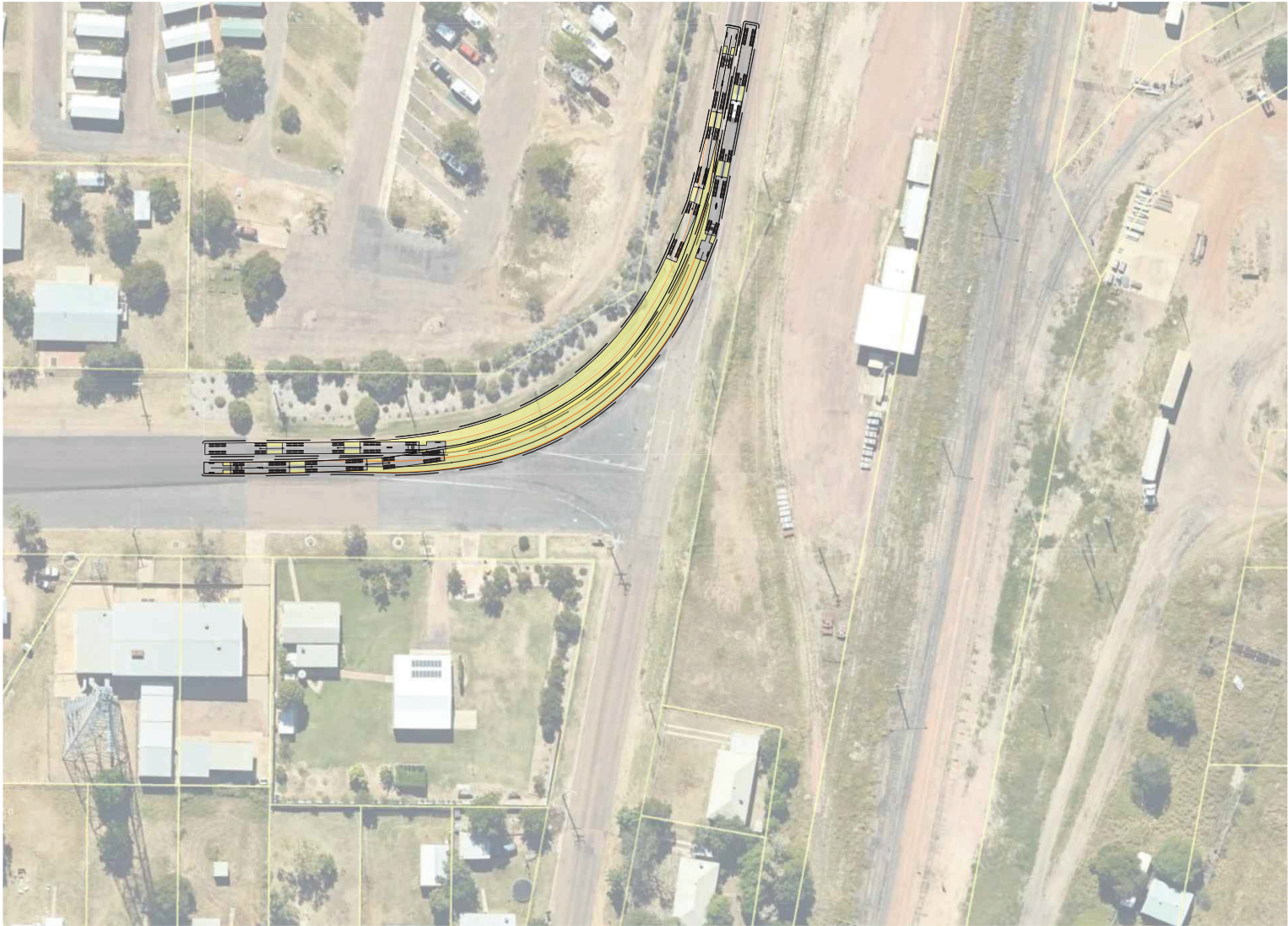
A TRIPLE SWEEP PATHS - TMR13 SCALE 1:500
