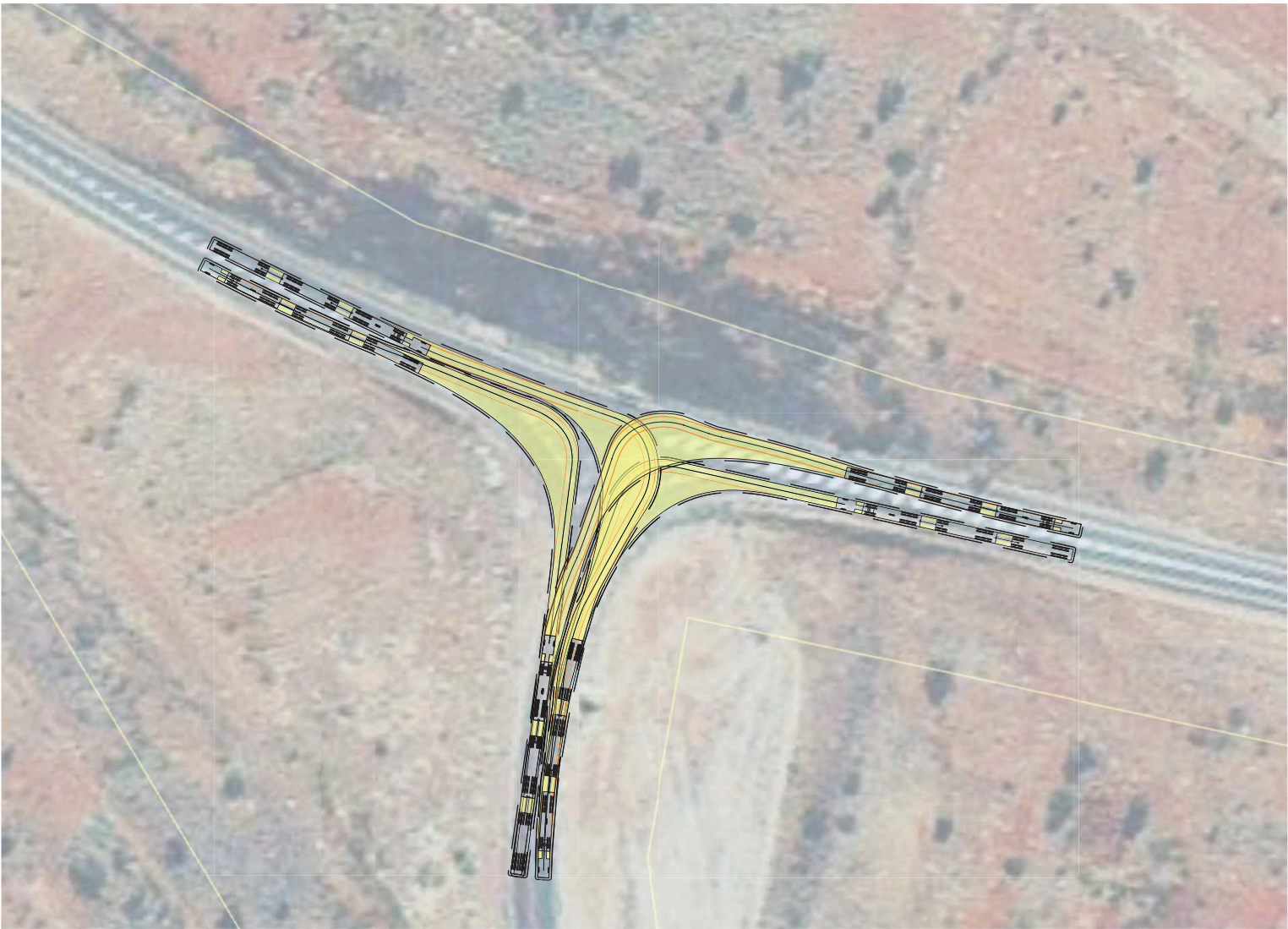
A TRIPLE SWEEP PATHS - TMR23 SCALE 1:500
