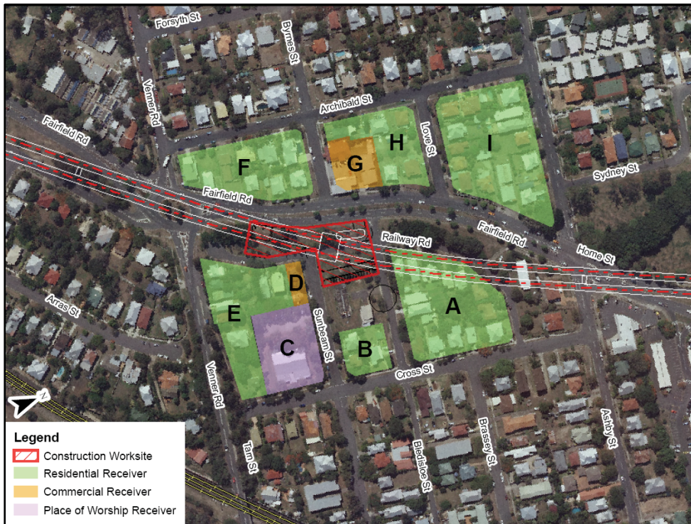
Figure 16-36 Ventilation and emergency access building and shaft worksite and receiver areas
