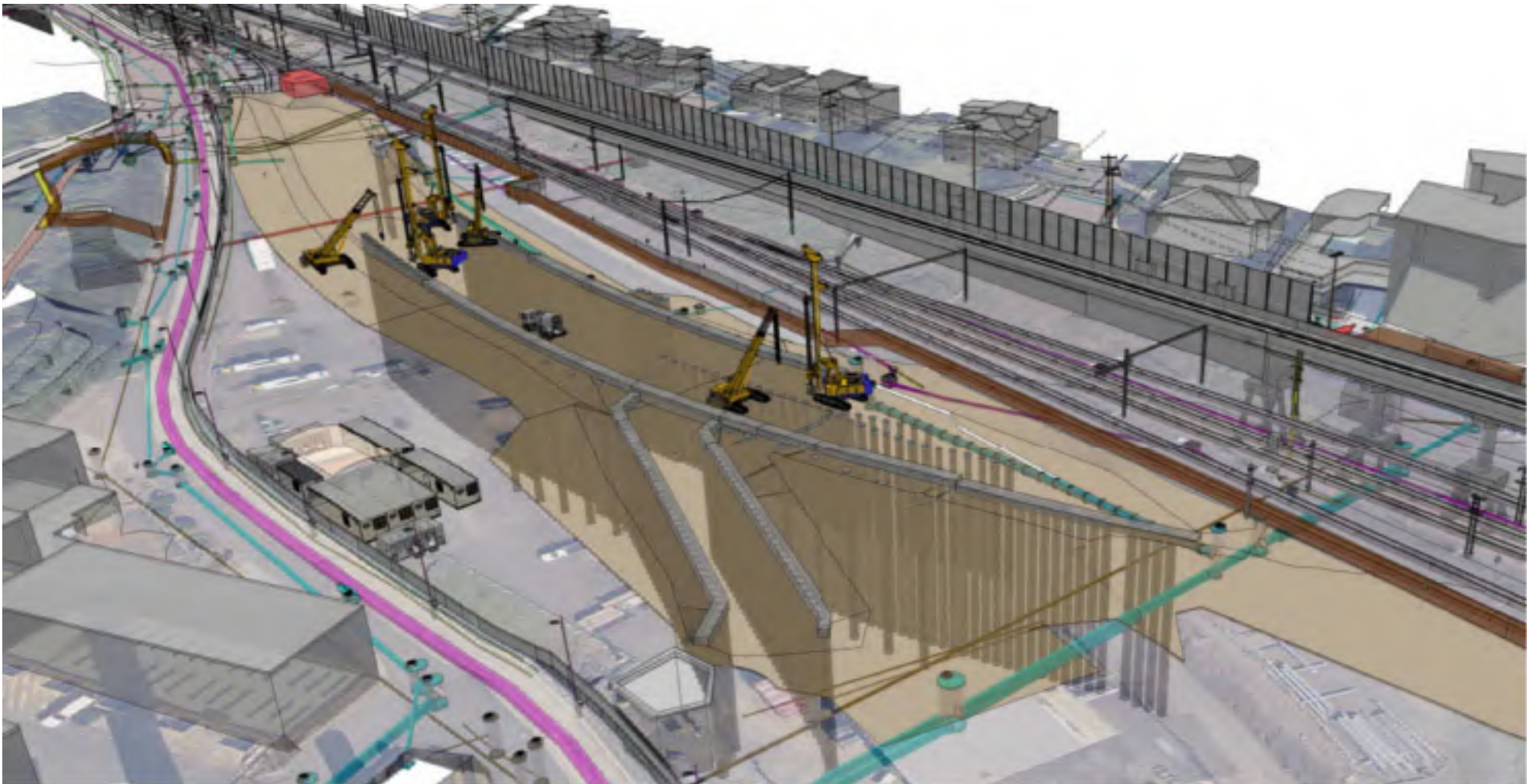
Figure C1.3: Stage 1 - 11 Months (construction works within Zone F)
