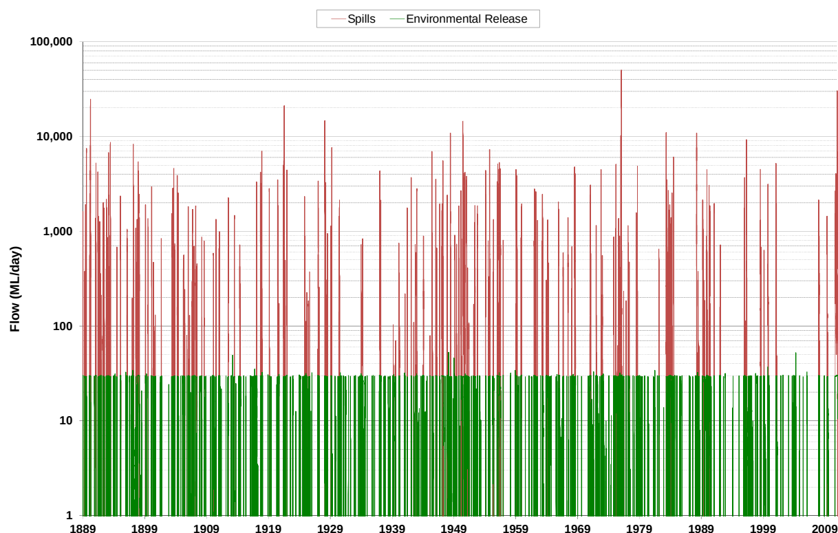
Figure A-1 Dam Release and Spills
