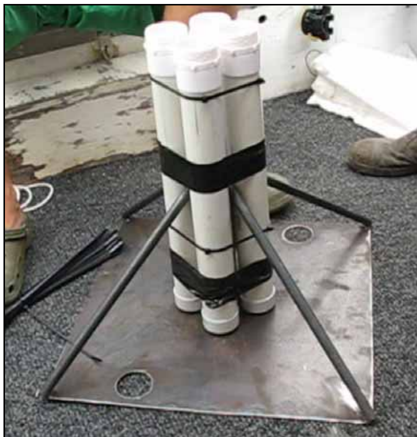
Figure 4-9 Typical Sediment Trap Assemblage
