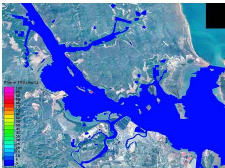
Figure 5-5 CSD with 50mg/L decant discharge – Plume snapshot at 01:00 on 18/02/2009 (Neap Tide)
