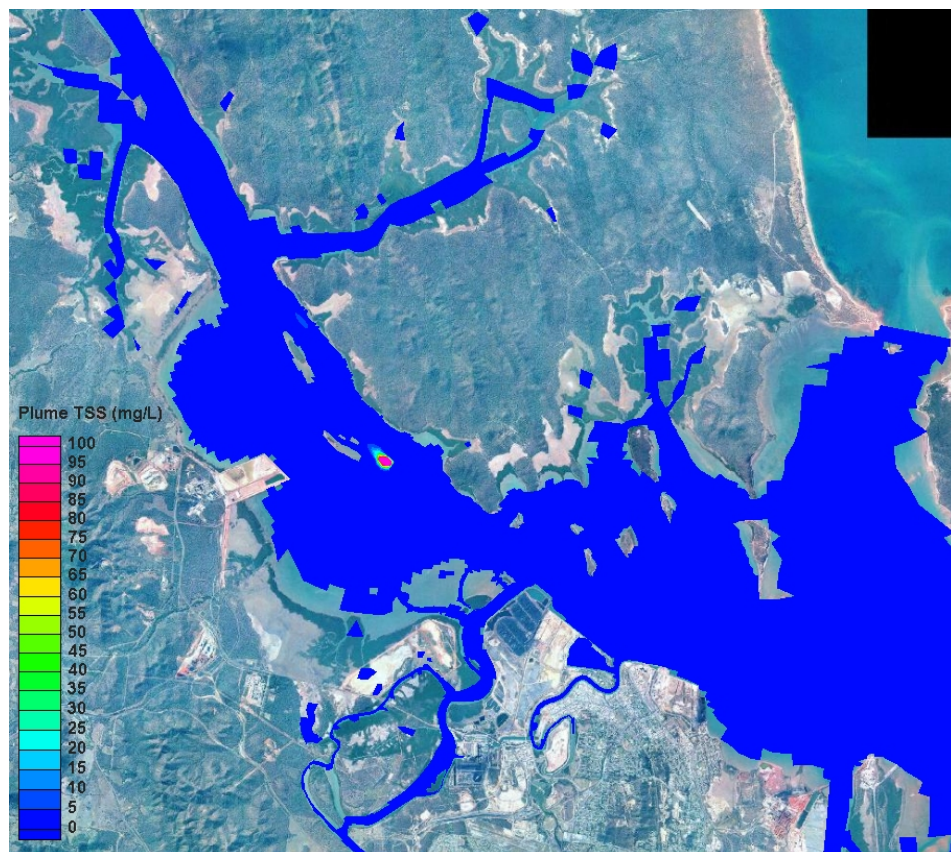
Figure 2-10 Scenario 1: CSD with 50mg/L decant - Plume snapshot at 01:00 on 18/02/2009
