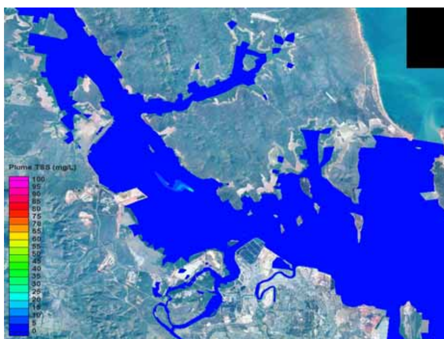
Figure 5-6 CSD with 50mg/L decant discharge – Plume snapshot at 09:00 on 26/02/2009 (Spring Tide)
