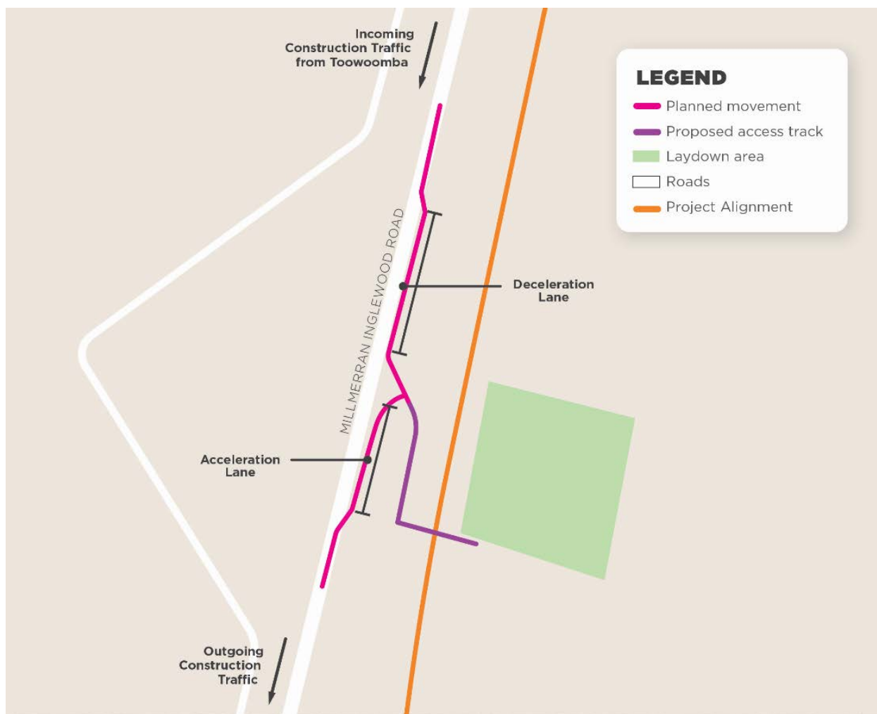
Figure 5.4 Typical construction traffic access to laydown area adjacent to DTMR road
