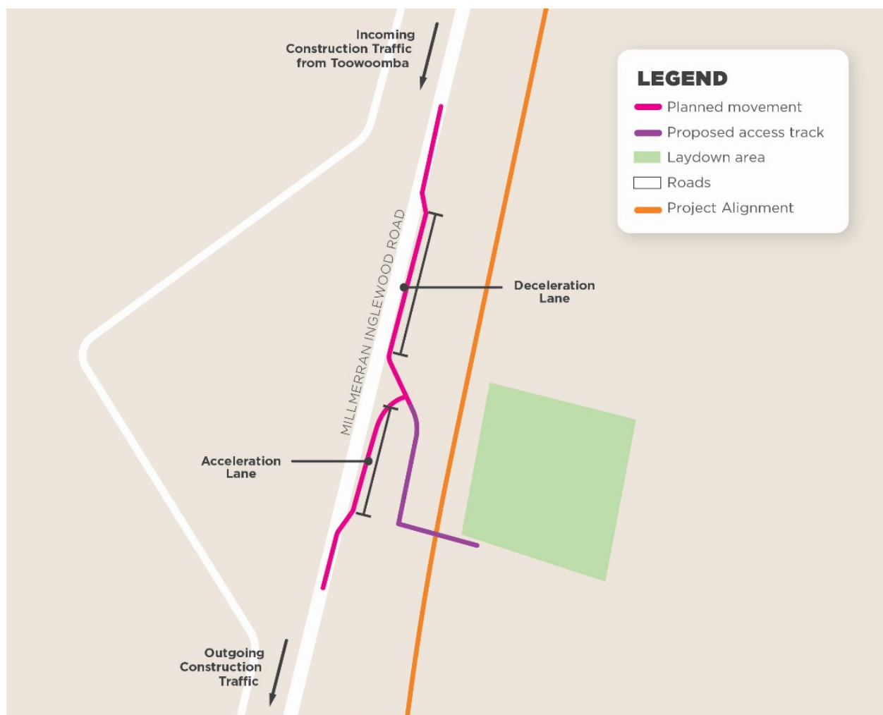
Figure 3.2 Typical construction traffic access to laydown area adjacent to State controlled roads
