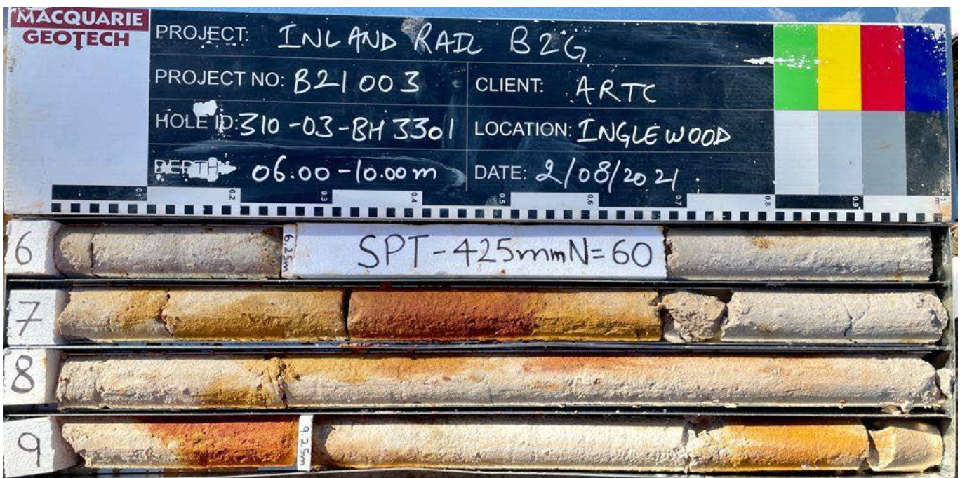
PointID : 310-03-BH3301 Depth Range: 6.00 - 10.00 m
