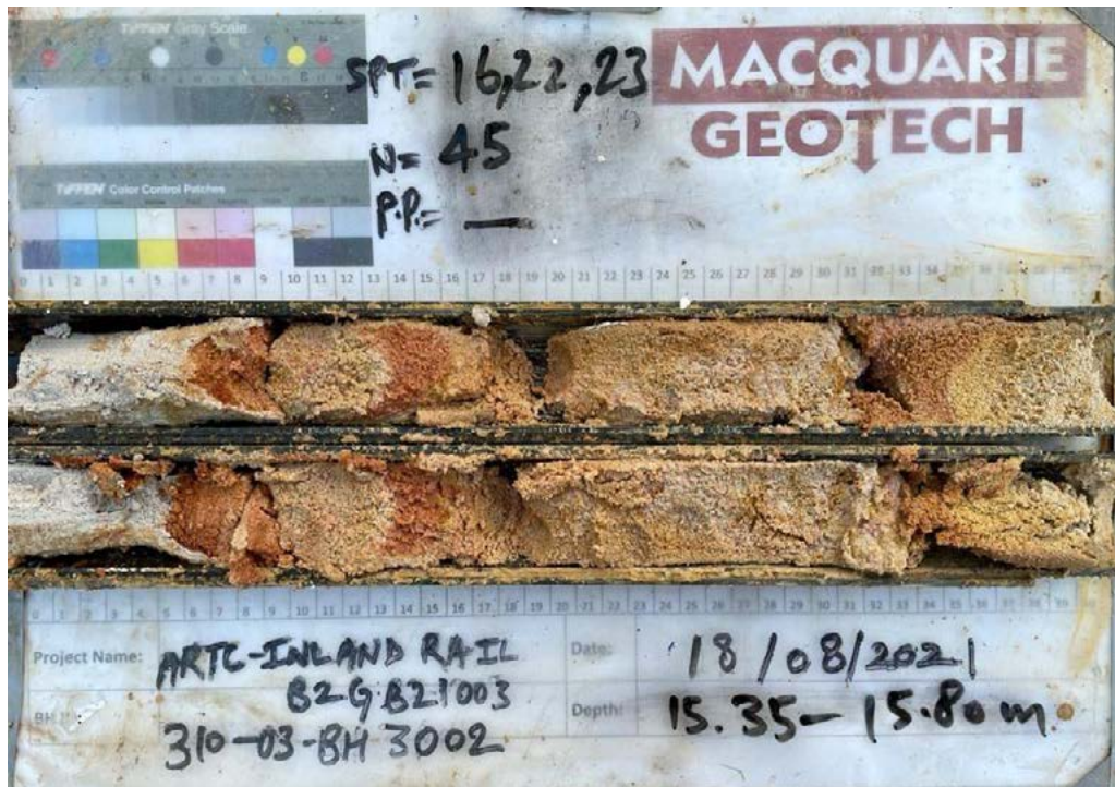
PointID : 310-03-BH3002 Depth Range: 15.35 - 15.80 m
