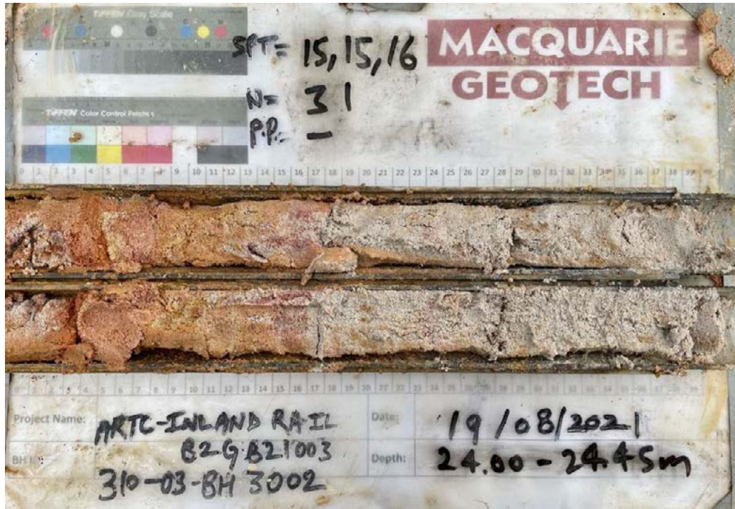
PointID : 310-03-BH3002 Depth Range: 24.00 - 24.45 m
