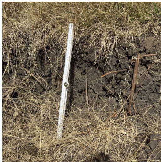
P10 – close up of erosion on true right bank downstream of pond. 0.5 m staff for scale (site E1)
