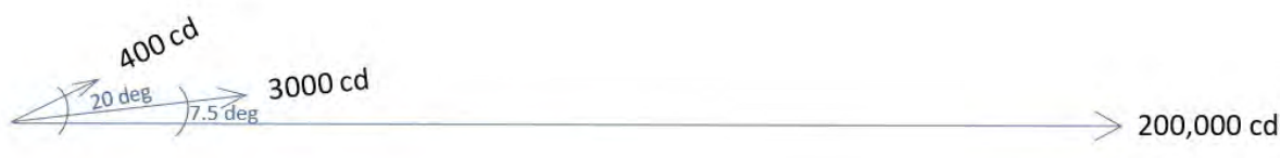
Figure 2.1 Australian standard requirements for headlights
