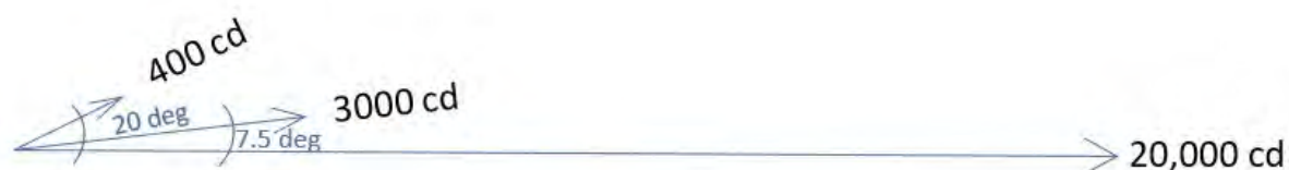
Figure 3.2 Australian standard requirements for visibility lighting
