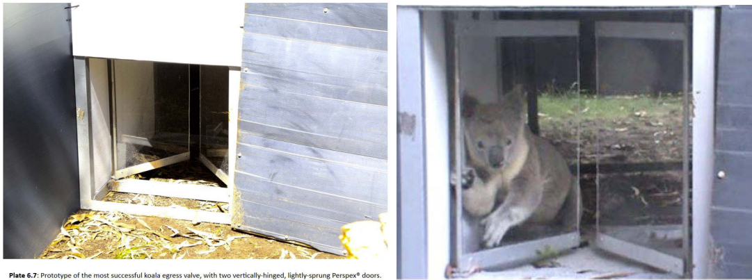
Figure 5.19 (Left) The design of a prototype of one-way gates for koalas, tested on captive animals as part of the Moreton Bay Rail Project. Koalas can push through the lightly-sprung doors at a 45° angle, but are (right photo) unable to pass through in the opposite direction (Hanger et al. 2017).
