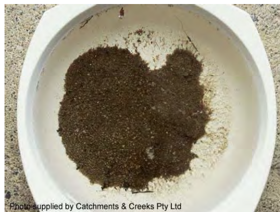
Photo 10 – Typical response of a slaking soil
