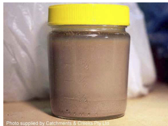
Photo 6 – Poor settlement indicates a high risk of dispersive properties
