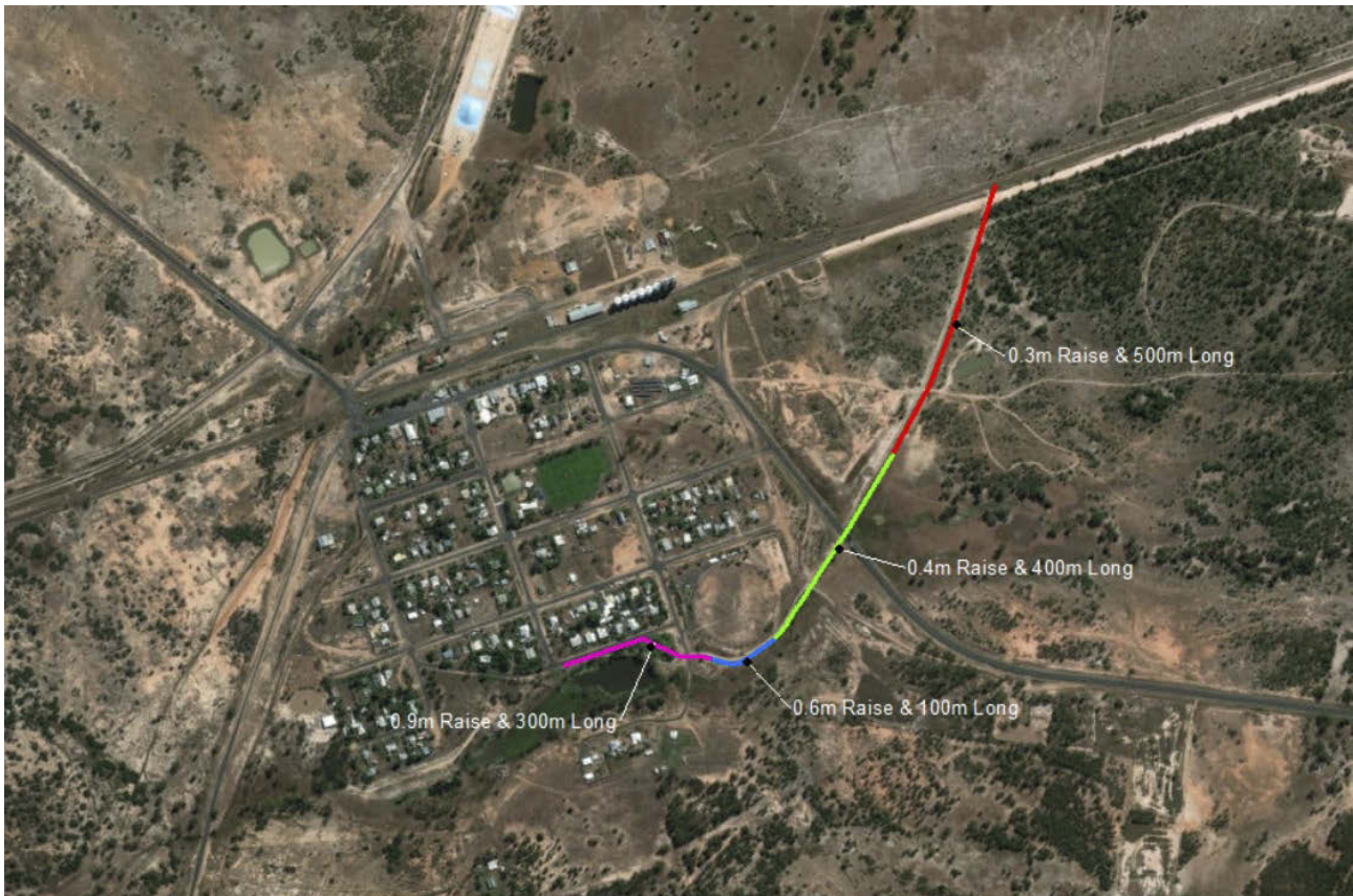
Figure 14.12 Yelarbon levee—Proposed raise heights
