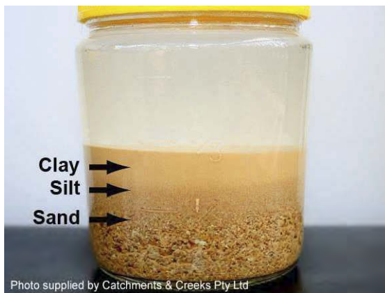
Photo 3 – Separate layers of clay, silt and sand visible in settled sample
