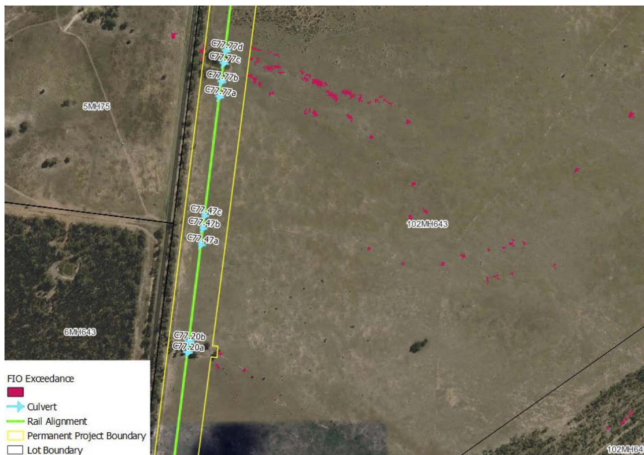
Figure 22.6 Site 2—Flood Impact Objective exceedances (post-mitigation)
