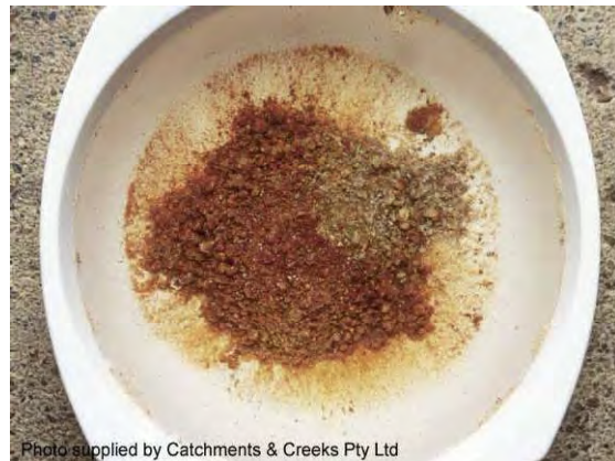
Photo 8 – Typical response of a slightly dispersive soil
