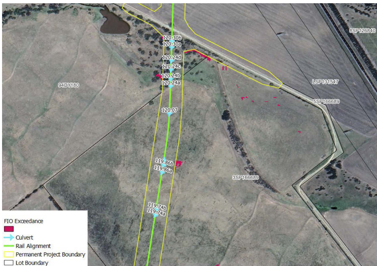
Figure 22.10 Site 4—Flood Impact Objective exceedances (post-mitigation)
