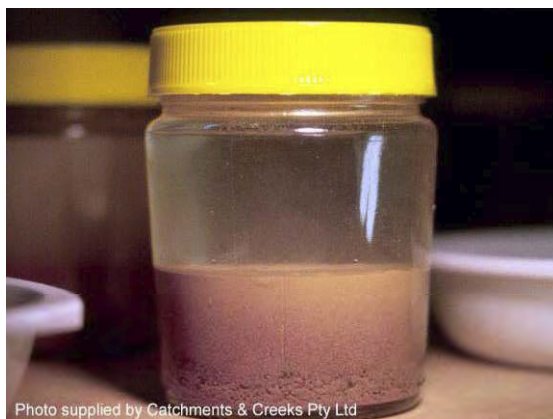
Photo 5 – Good settlement indicates soil is unlikely dispersive
