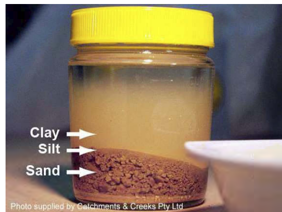
Photo 4 – Slow settlement after 1-day indicates a very fine clay
