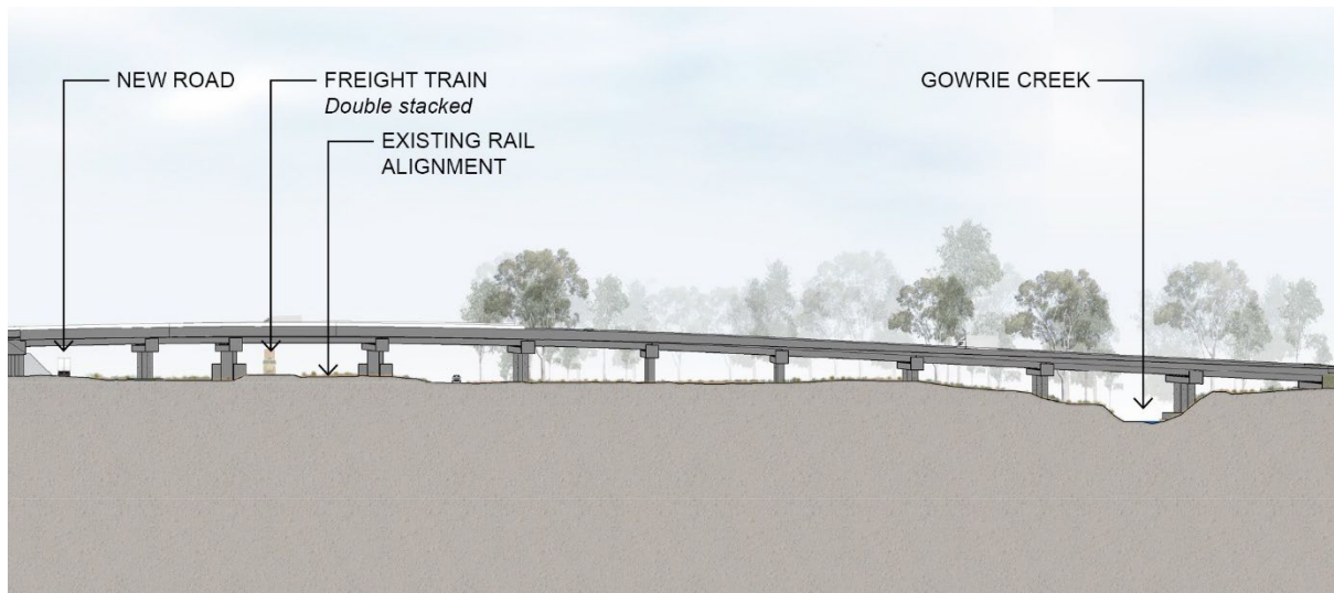
Figure 23: Gowrie Junction Road bridge indicative elevation
