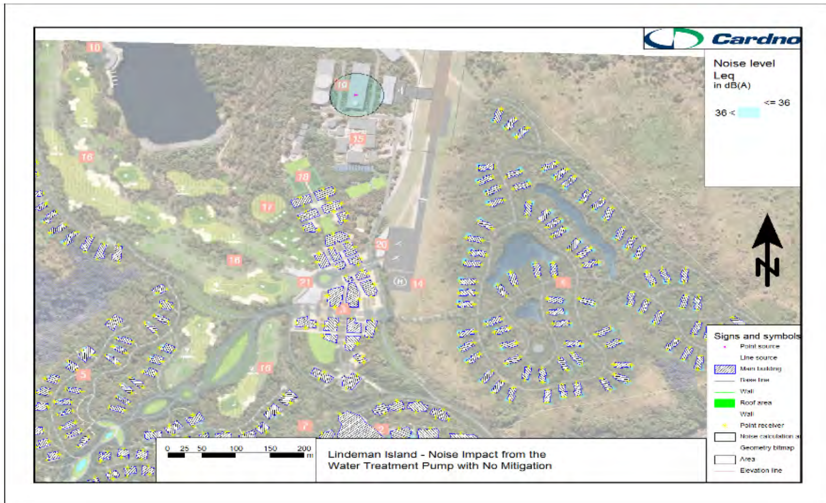
Figure 27 Predicted Noise Impact – Water Treatment Pump
