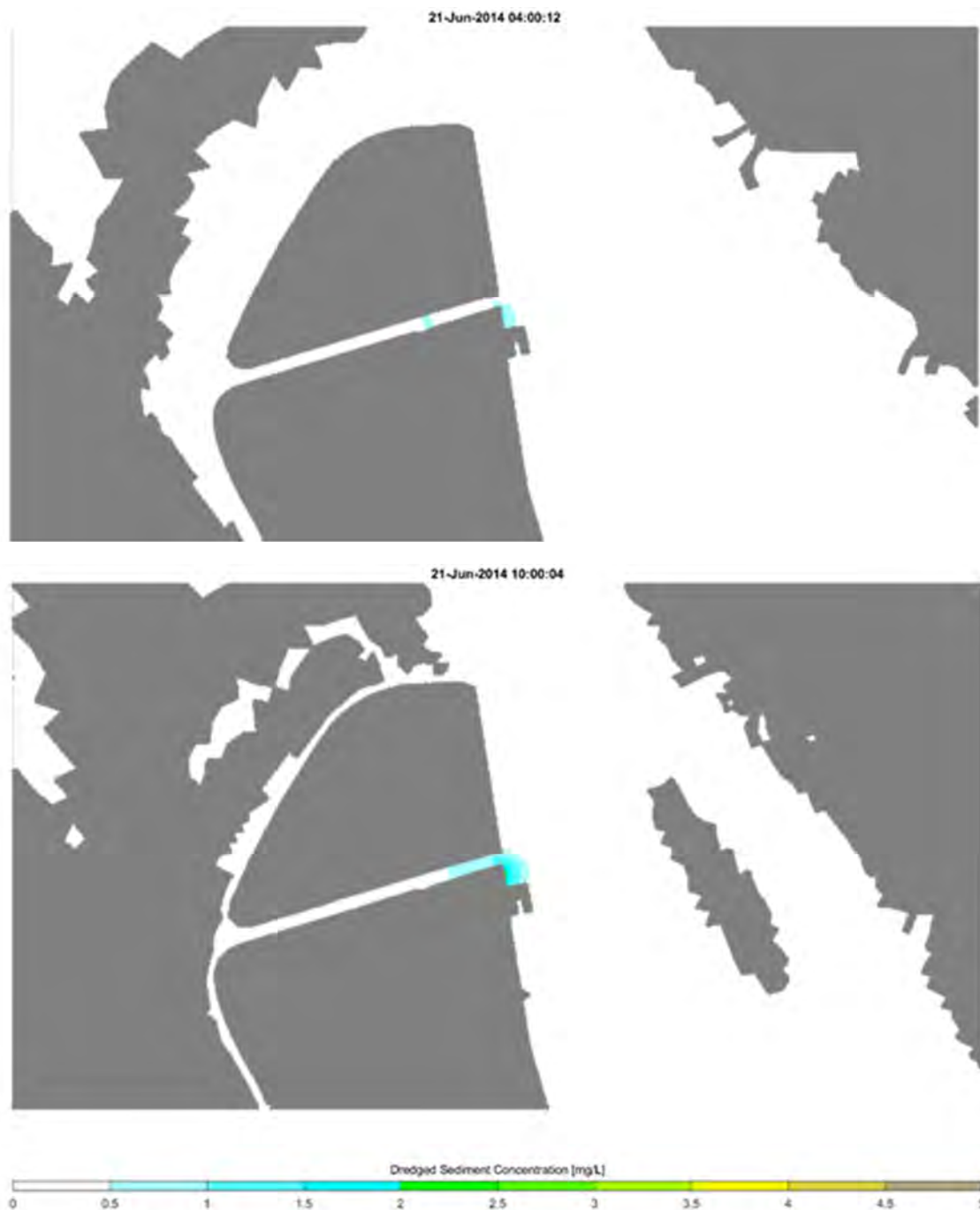
Figure 5-31 Typical Tailwater Plume Depth-Average TSS Concentration (Top: Neap Flood Tide, Bottom: Neap Ebb Tide)
