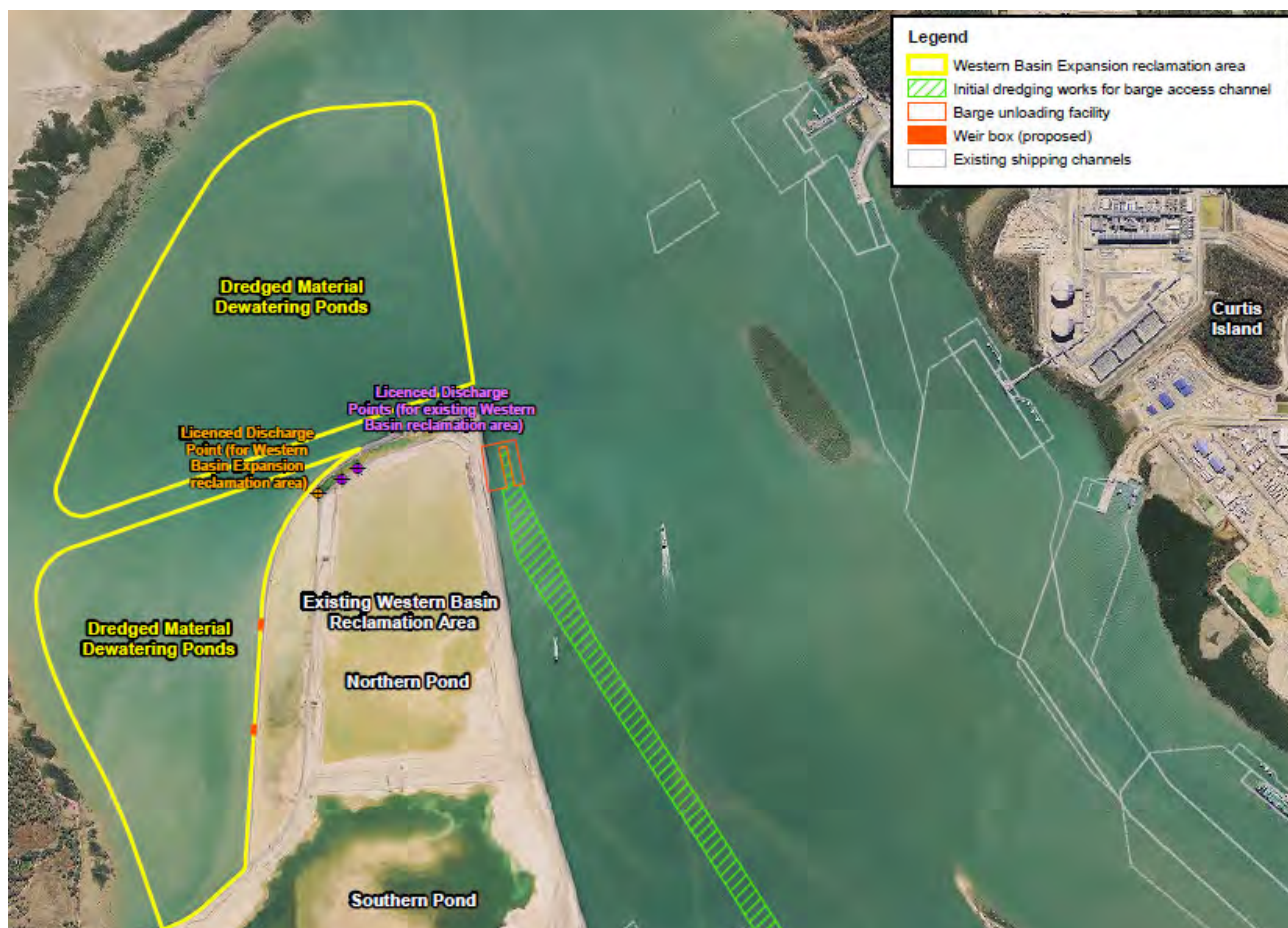
Figure 5-4 Project Tailwater Discharge Locations
