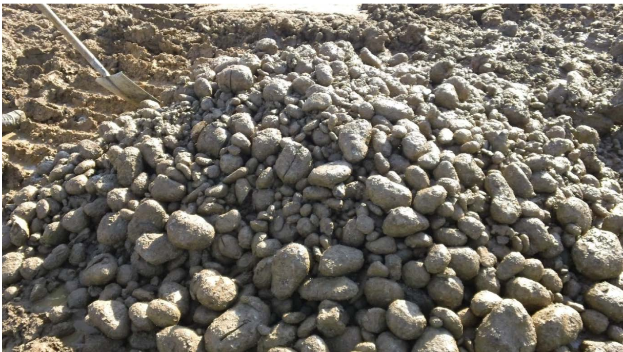
Figure 4.5 Dredged material forming clay balls from the Western Basin Project
