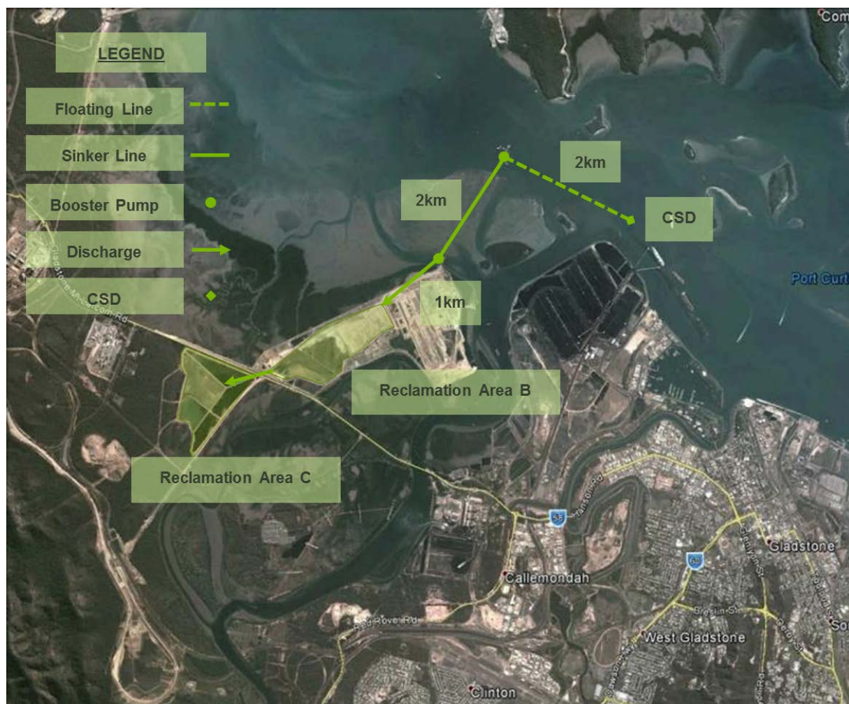
Figure 5.1 WICT Project dredging and reclamation infrastructure placement arrangement
