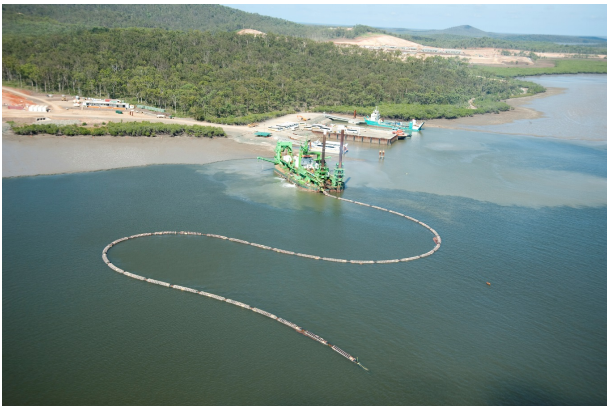
Figure 4.1 The 'Al Mahaar' CSD operating in the Port of Gladstone
