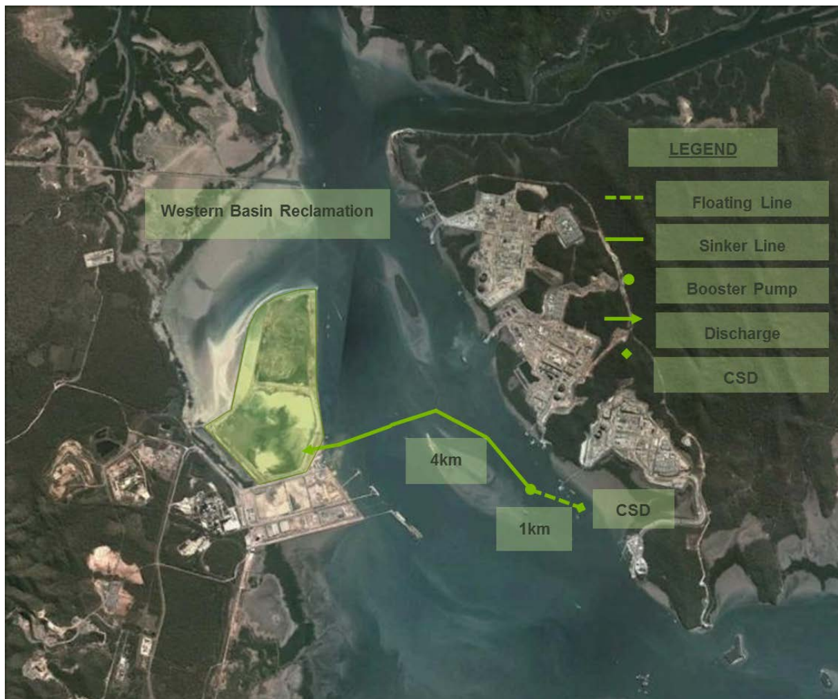
Figure 5.5 Western Basin Project dredging and intertidal reclamation arrangement
