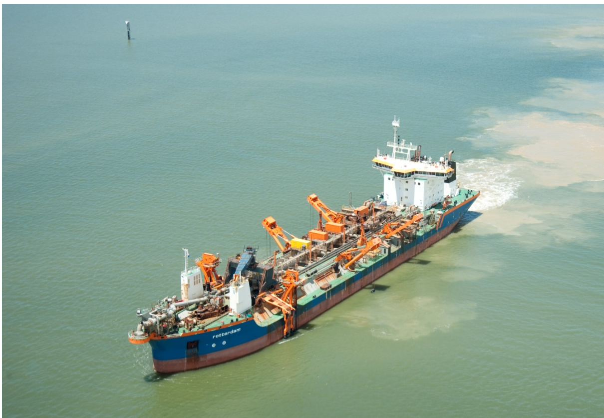
Figure 4.2 The 'Rotterdam' TSHD operating within the Port of Gladstone
