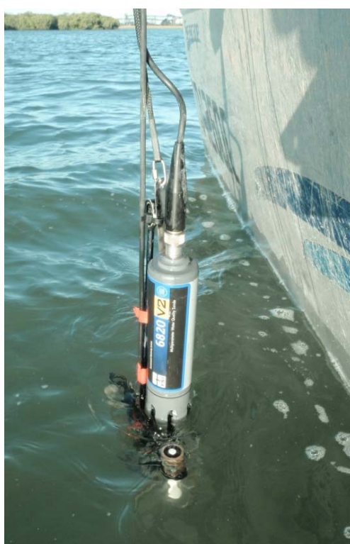
Photograph 2.5 Measurement of physicochemical parameters
