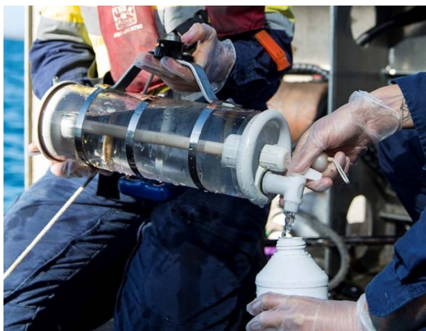
Photograph 2.7 Collection of water samples for analysis using the Van Dorn sampler
