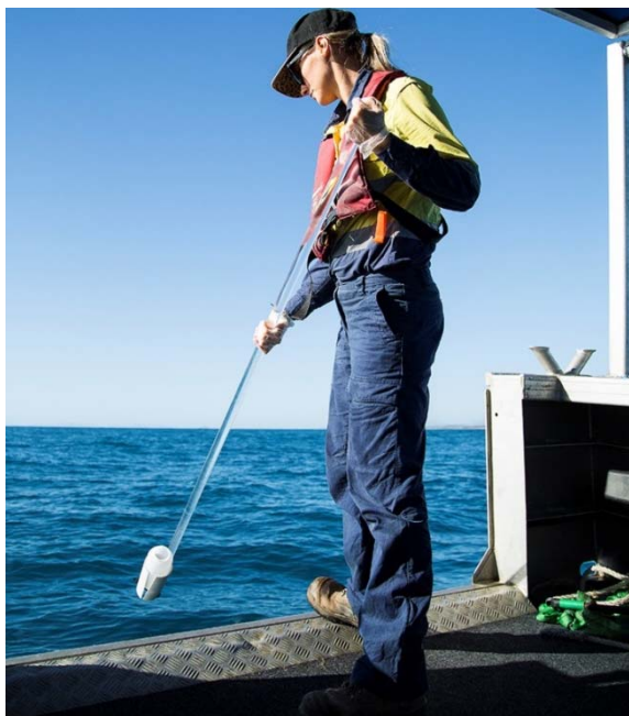
Photograph 2.6 Collection of water samples for analysis using Perspex Pole sampler
