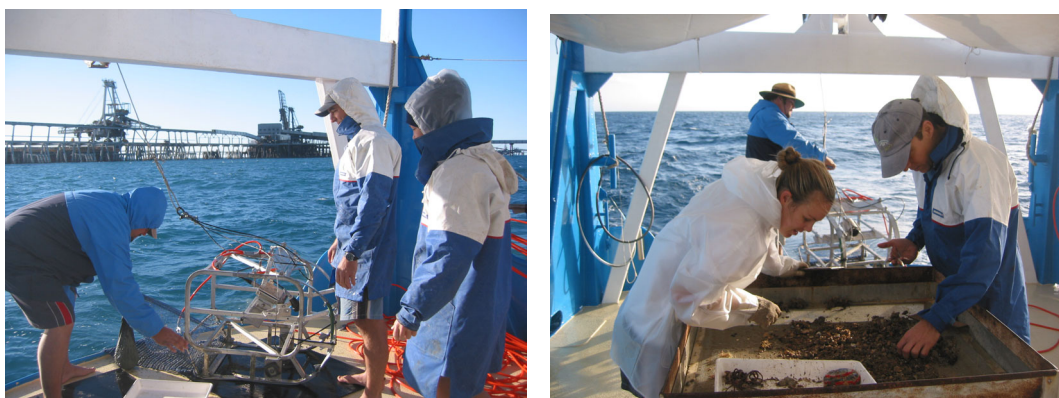
Plate 1 Offshore video sampling sled and sorting benthic samples from the sled net.
