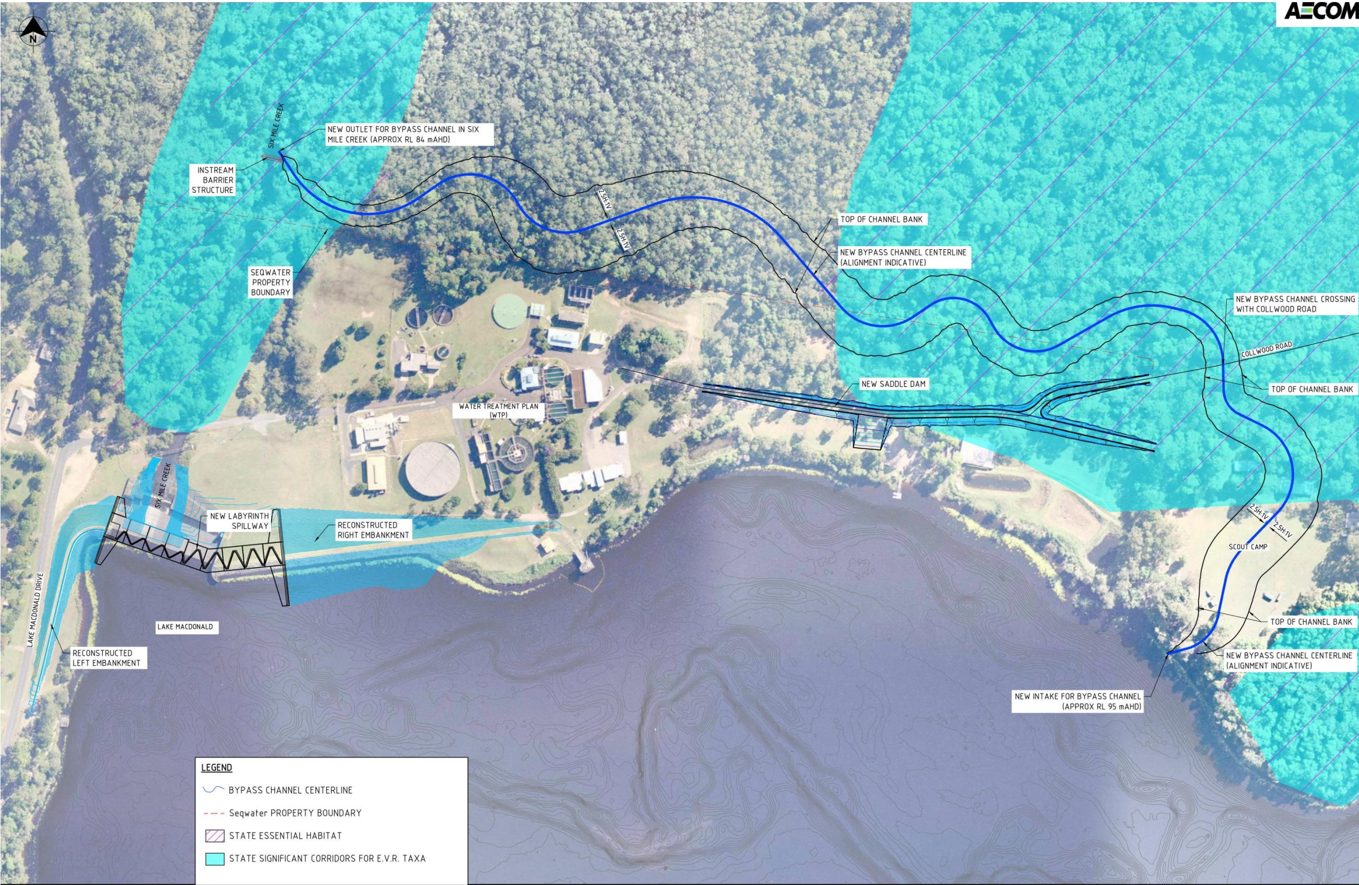
Figure 6 Potential layout for bypass channel fishway
