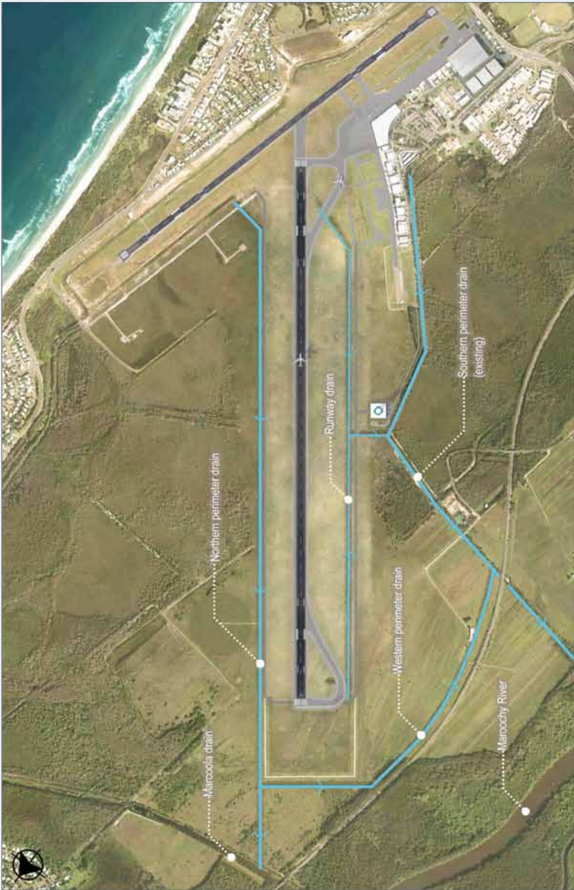
Figure 5.1g: Proposed drainage infrastructure
