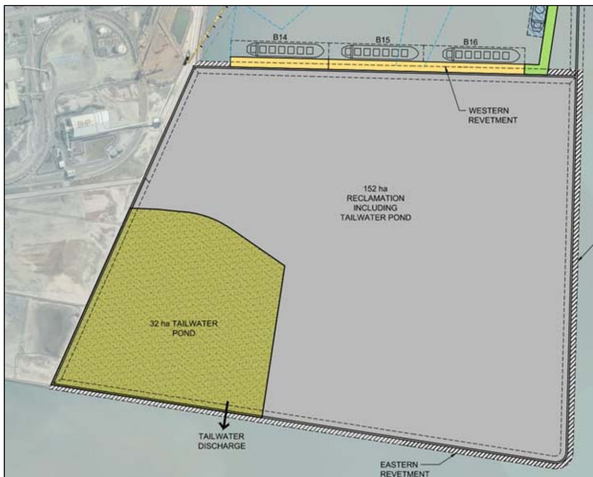
Figure 6.21 Tailwater Discharge Location from the Reclamation Area
