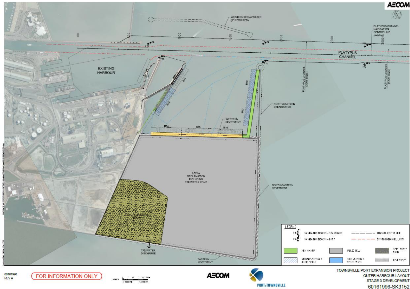
Figure 1-2 Port Expansion Staging and Geometry – Stages 2 and 3
