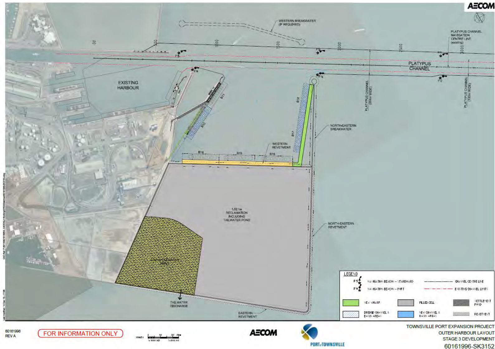
Figure 1-2 Port Expansion Staging and Geometry – Stages 2 and 3
