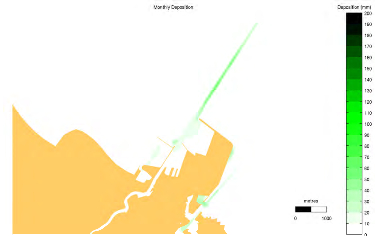
Figure 5-6 Modelled Ultimate Case Siltation Rate (mm/month)
