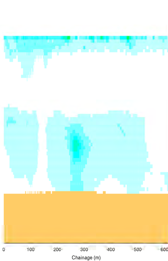
ADCP Dredge Plume in Profile
