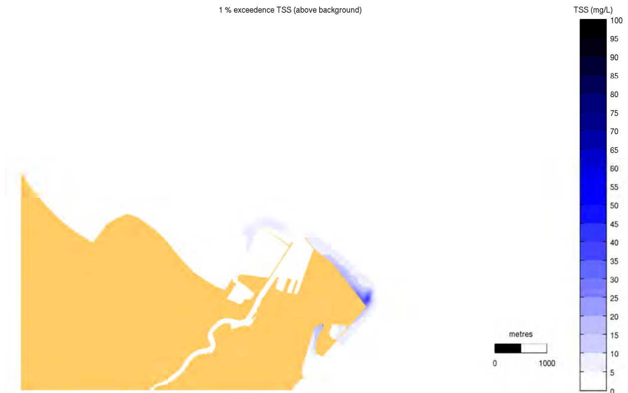
Figure 6-6 Scenario 2a - Above Background Total Suspended Sediment Concentration (mg/L) Exceeded for 1% of the Simulation Period
