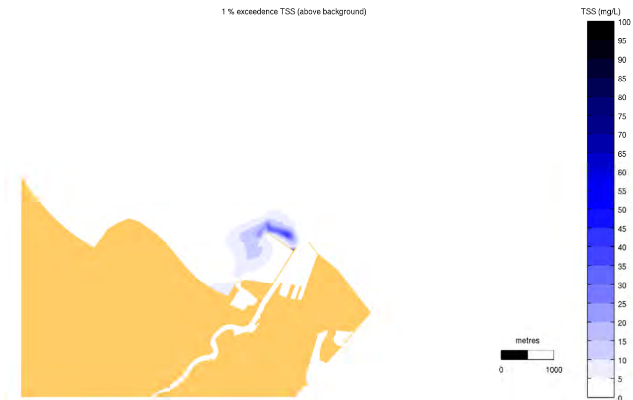
Figure 6-3 Scenario 1b - Above Background Suspended Sediment Concentration (mg/L) Exceeded for 1% of the Simulation Period
