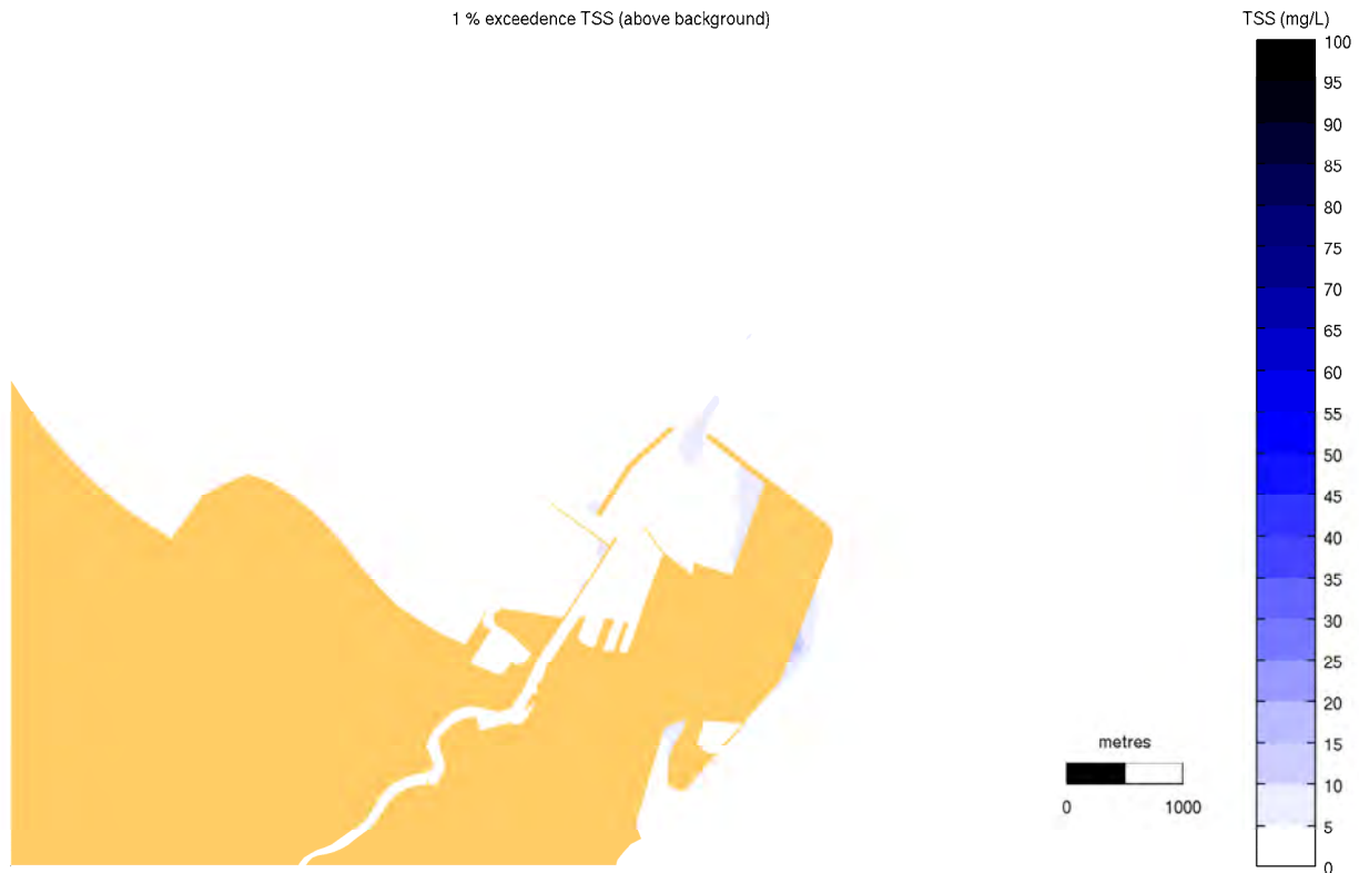
Figure 6-16 Scenario 4d - Above Background Total Suspended Sediment Concentration (mg/L) Exceeded for 1% of the Simulation Period
