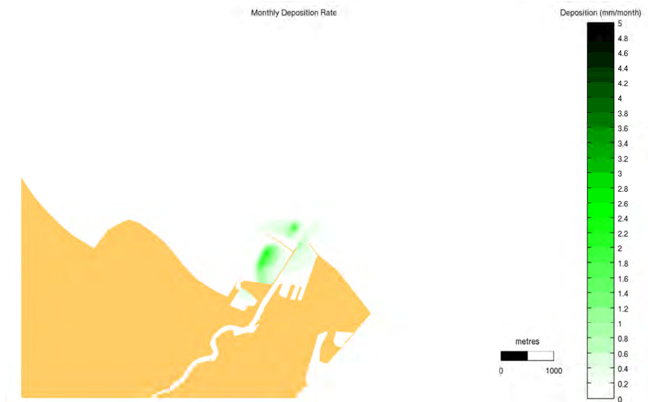
Figure 6-9 Scenario 2b – Modelled Sediment Deposition Rate (mm/month)
