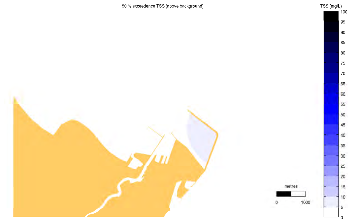
Figure 6-12 Scenario 3a - Above Background Total Suspended Sediment Concentration (mg/L) Exceeded for 50% of the Simulation Period
