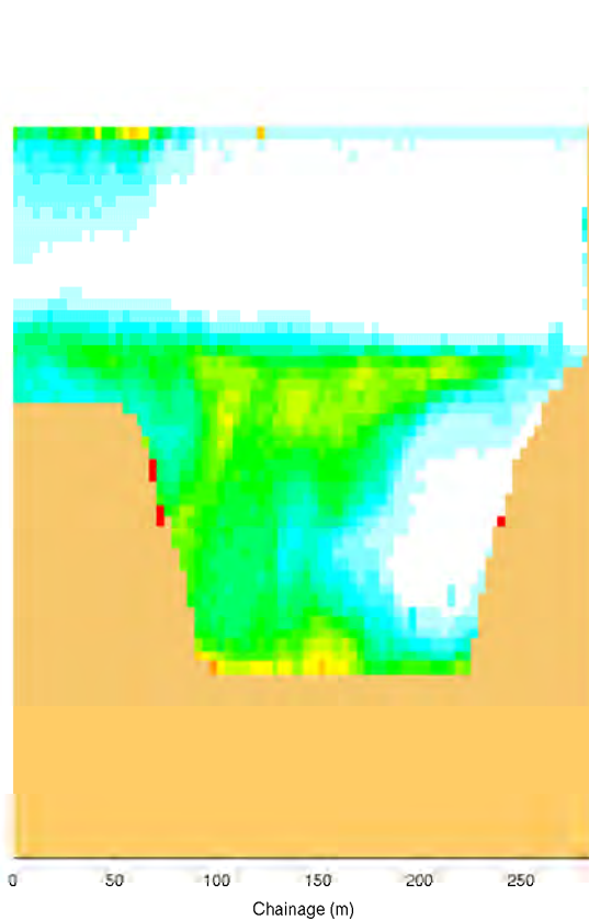
ADCP Dredge Plume in Profile
