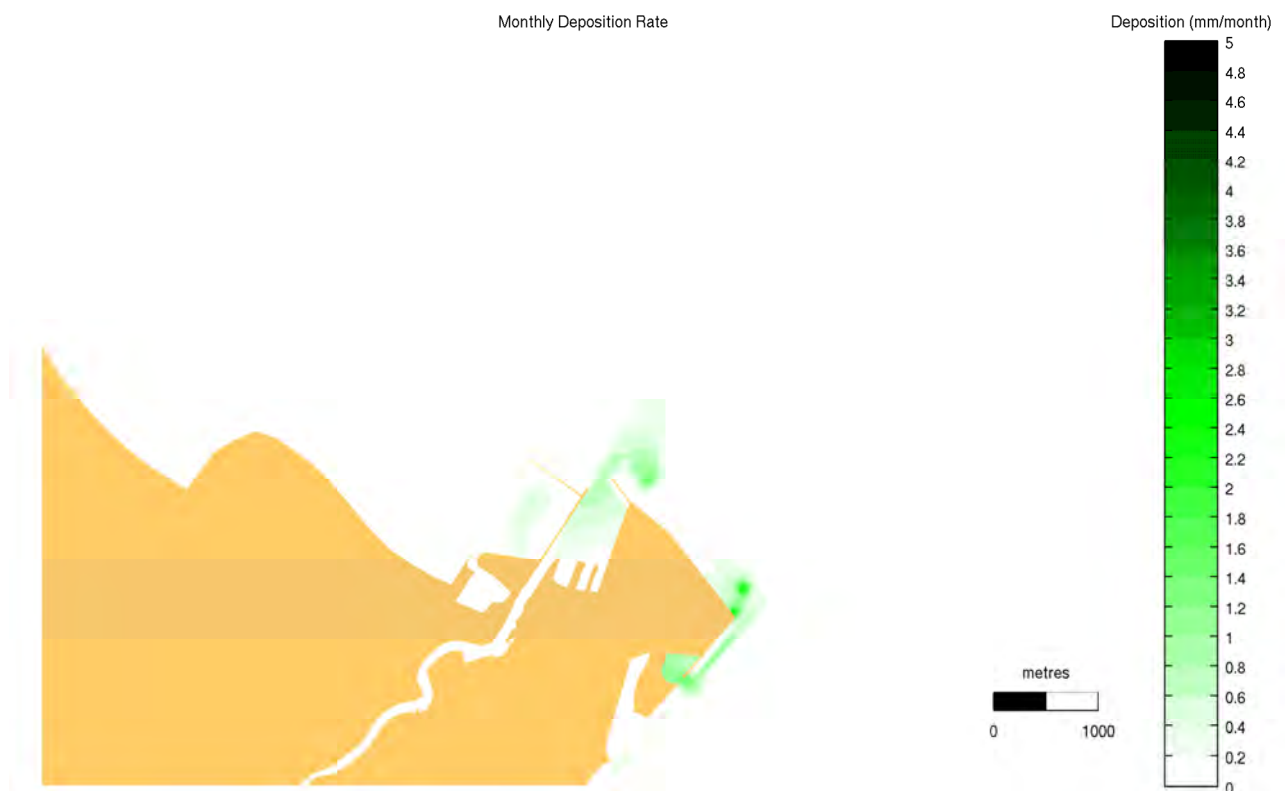
Figure 6-8 Scenario 2a – Modelled Sediment Deposition Rate (mm/month)
