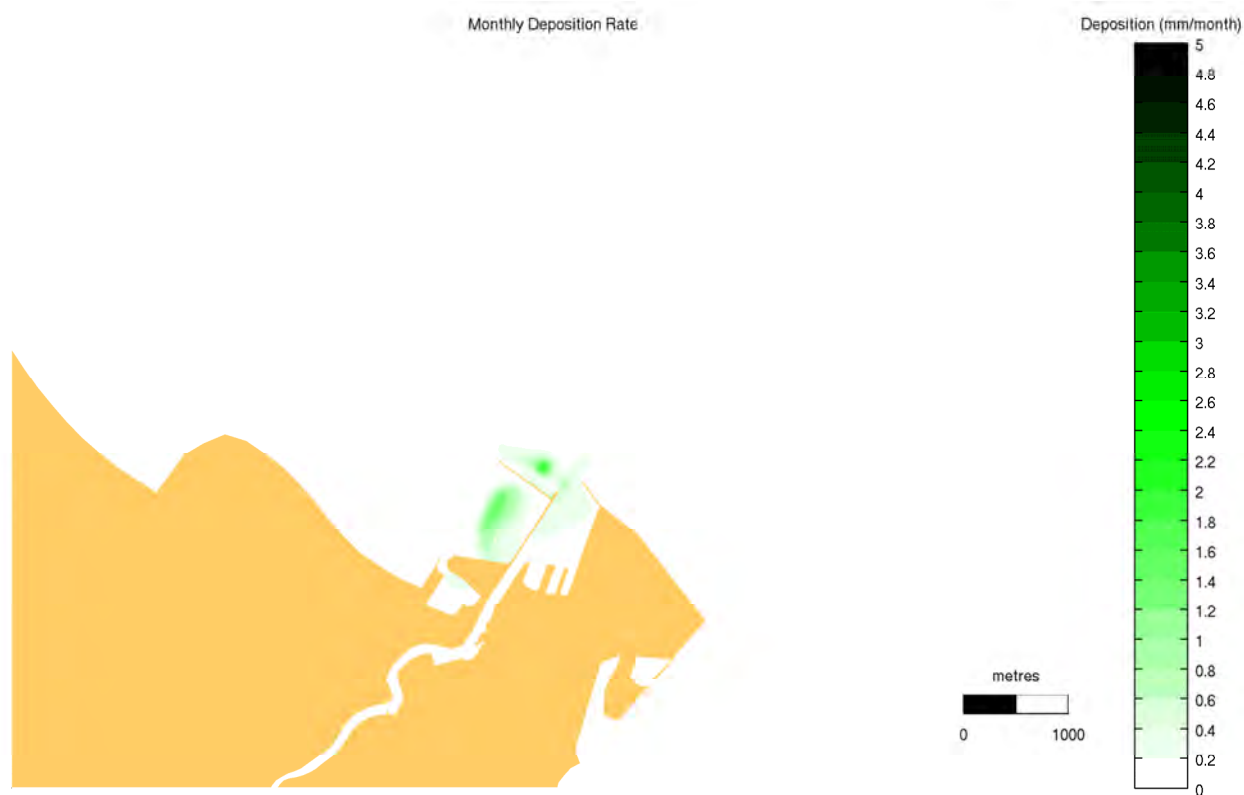
Figure 6-4 Scenario 1a – Modelled Sediment Deposition Rate (mm/month)
