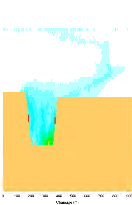
ADCP Dredge Plume in Profile
