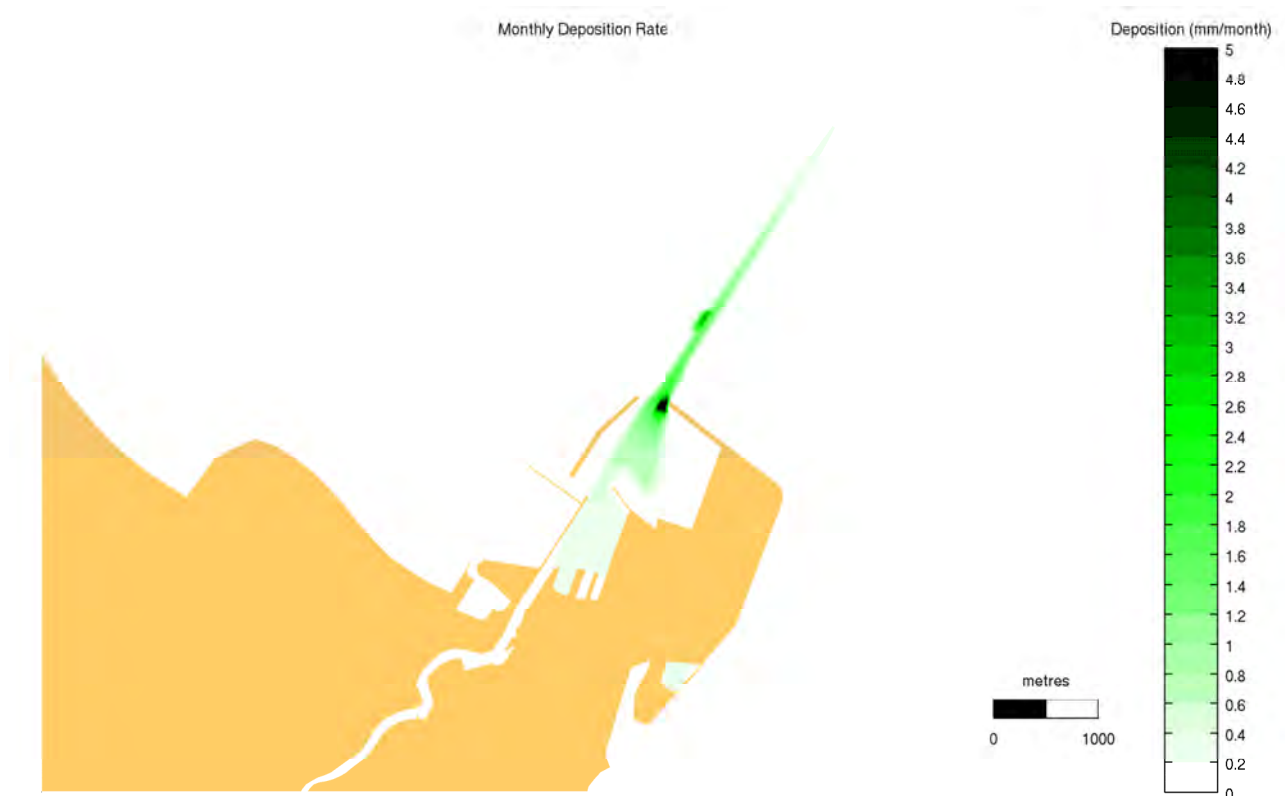
Figure 6-17 Scenario 4d – Modelled Sediment Deposition Rate (mm/month)
