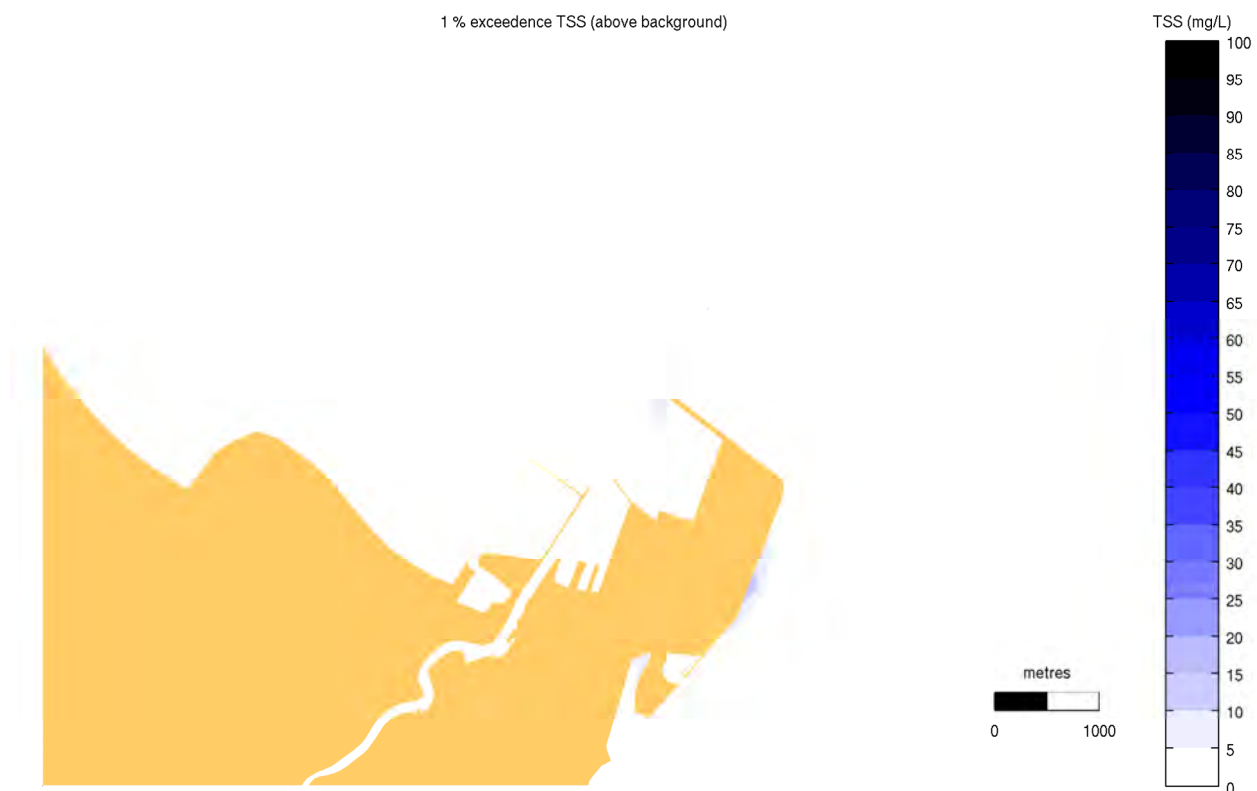
Figure 6-14 Scenario 4c - Above Background Total Suspended Sediment Concentration (mg/L) Exceeded for 1% of the Simulation Period
