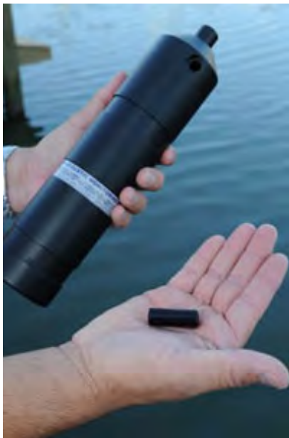
Figure 2-4 VR2W receiver and tag
