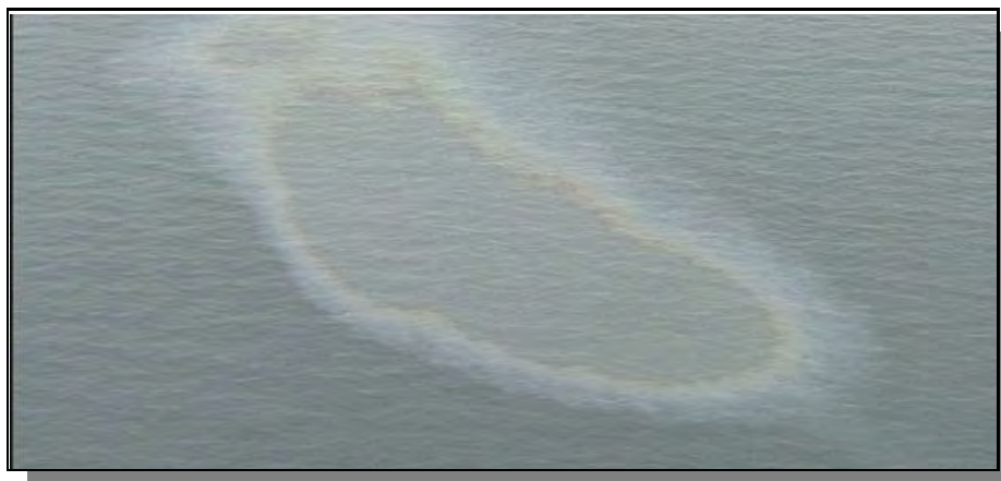
Figure 5: A photograph showing the difference between metallic appearance in the centre and the silvery and rainbow sheen oil around the edges. The thickness of the metallic is between 5 \mu\text{m} - 50 \mu\text{m} ; rainbow sheen is between 0.3 \mu\text{m} – 5.0 \mu\text{m} ; and silvery sheen is between 0.04 \mu\text{m} – 0.3 \mu\text{m} . The thickness of the (source: Bonn Agreement Aerial Surveillance Handbook, 2004 – Part 3, Annex A).
